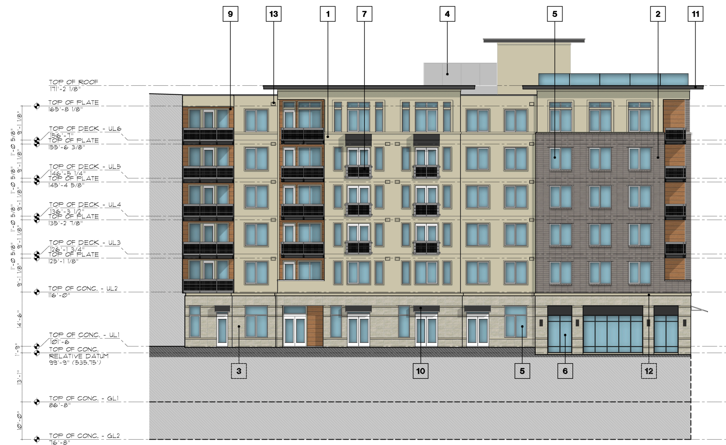
03 INTERIOR COURTYARD SOUTH ELEVATION SCALE: 1/16" = 1'-0"
