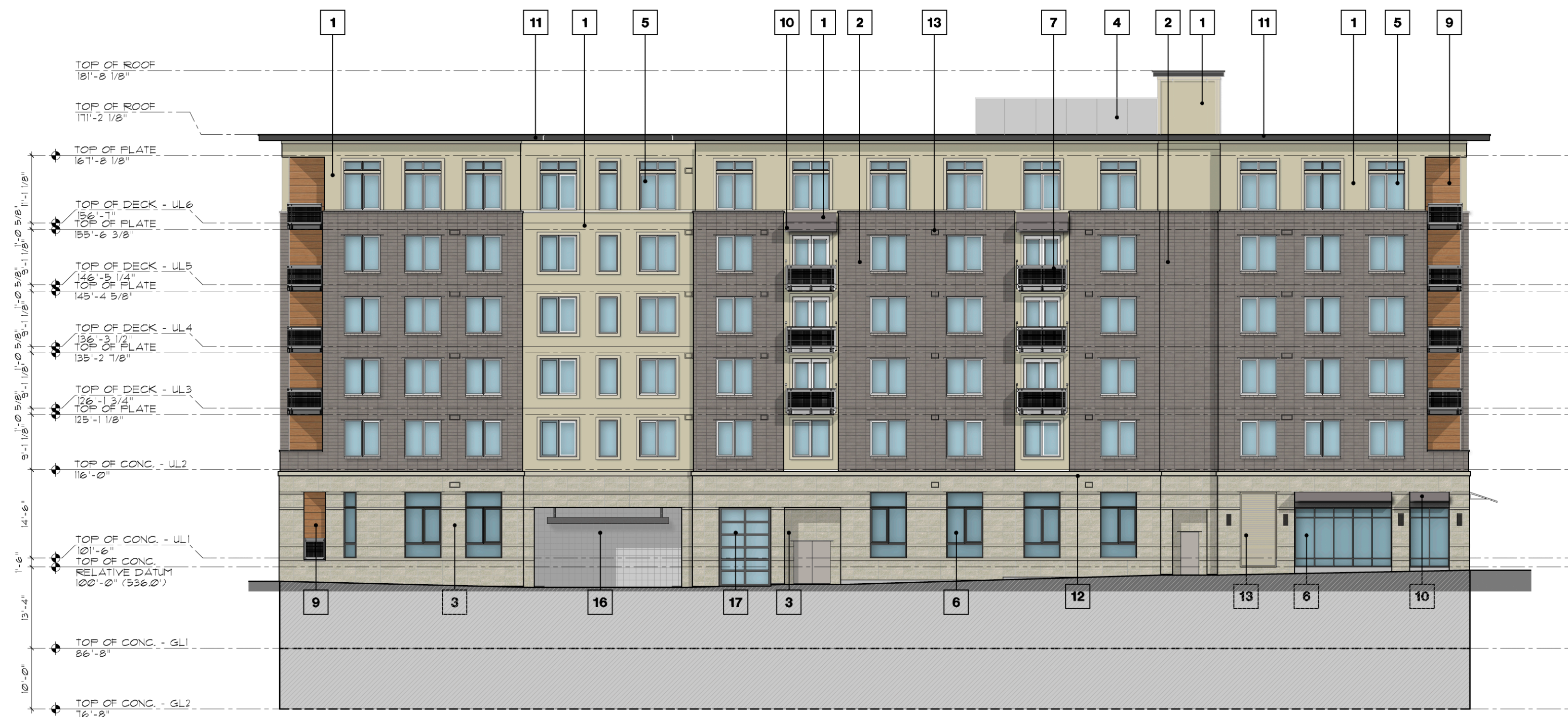
01 SOUTH ELEVATION 3.W. ABERNETHY SCALE: 1/16" = 1'-0"
