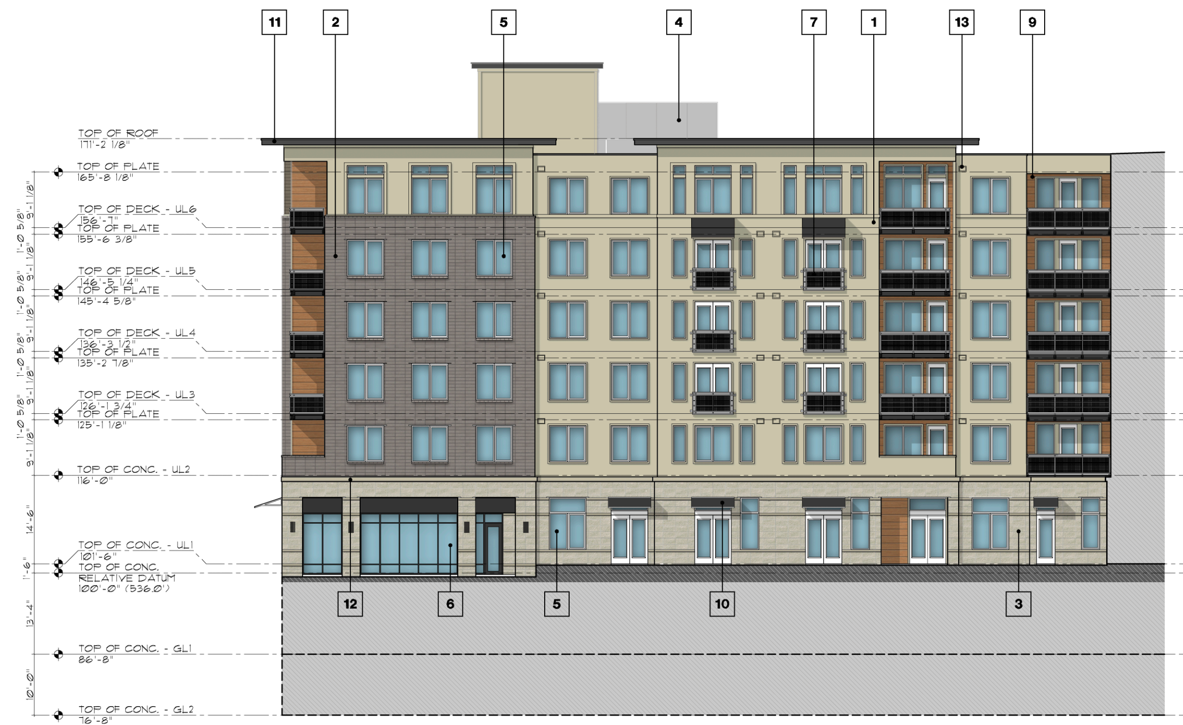
02 INTERIOR COURTYARD NORTH ELEVATION SCALE: 1/16" = 1'-0"
