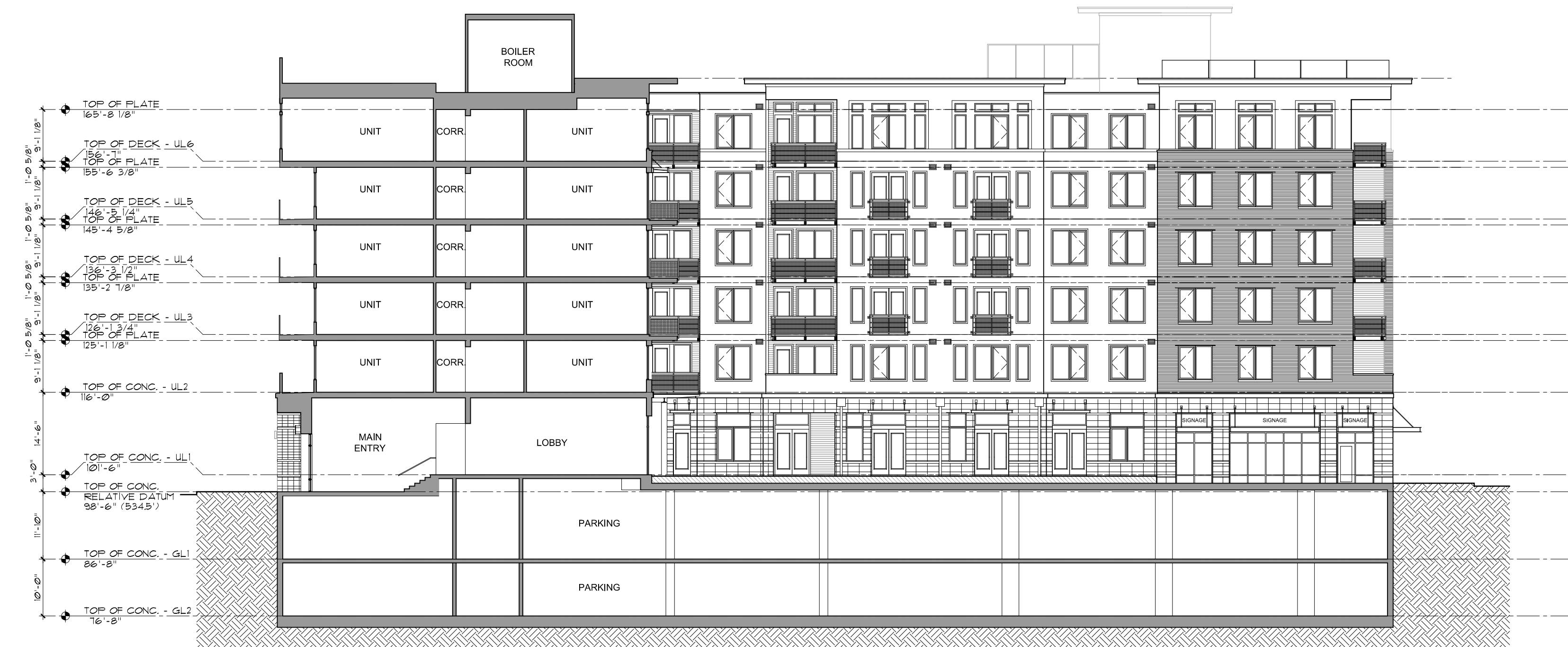
01 WEST-EAST SECTION AT COURTYARD SCALE: 1/16" = 1'-0"
