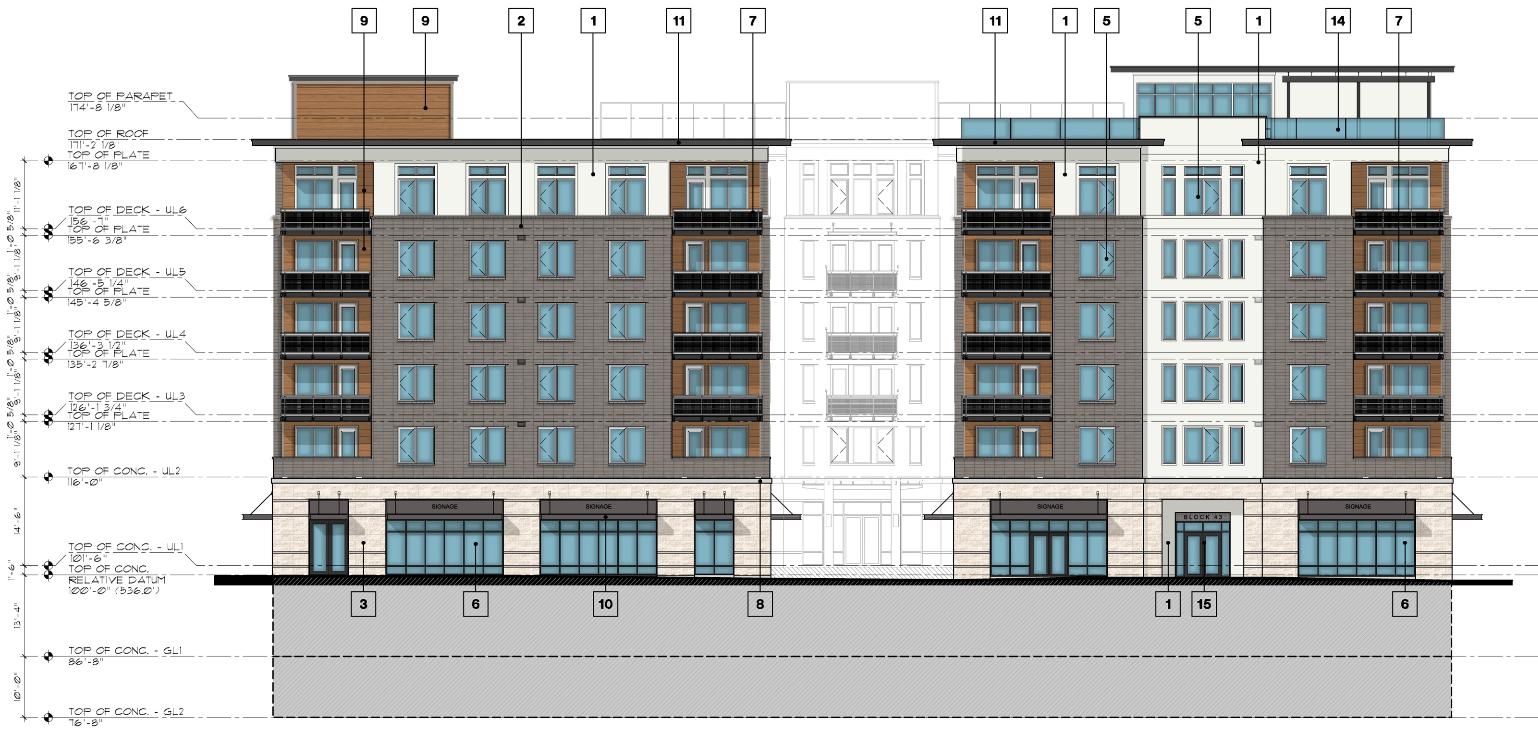
02 EAST ELEVATION S.W. BOND SCALE: 1/16" = 1'-0"
