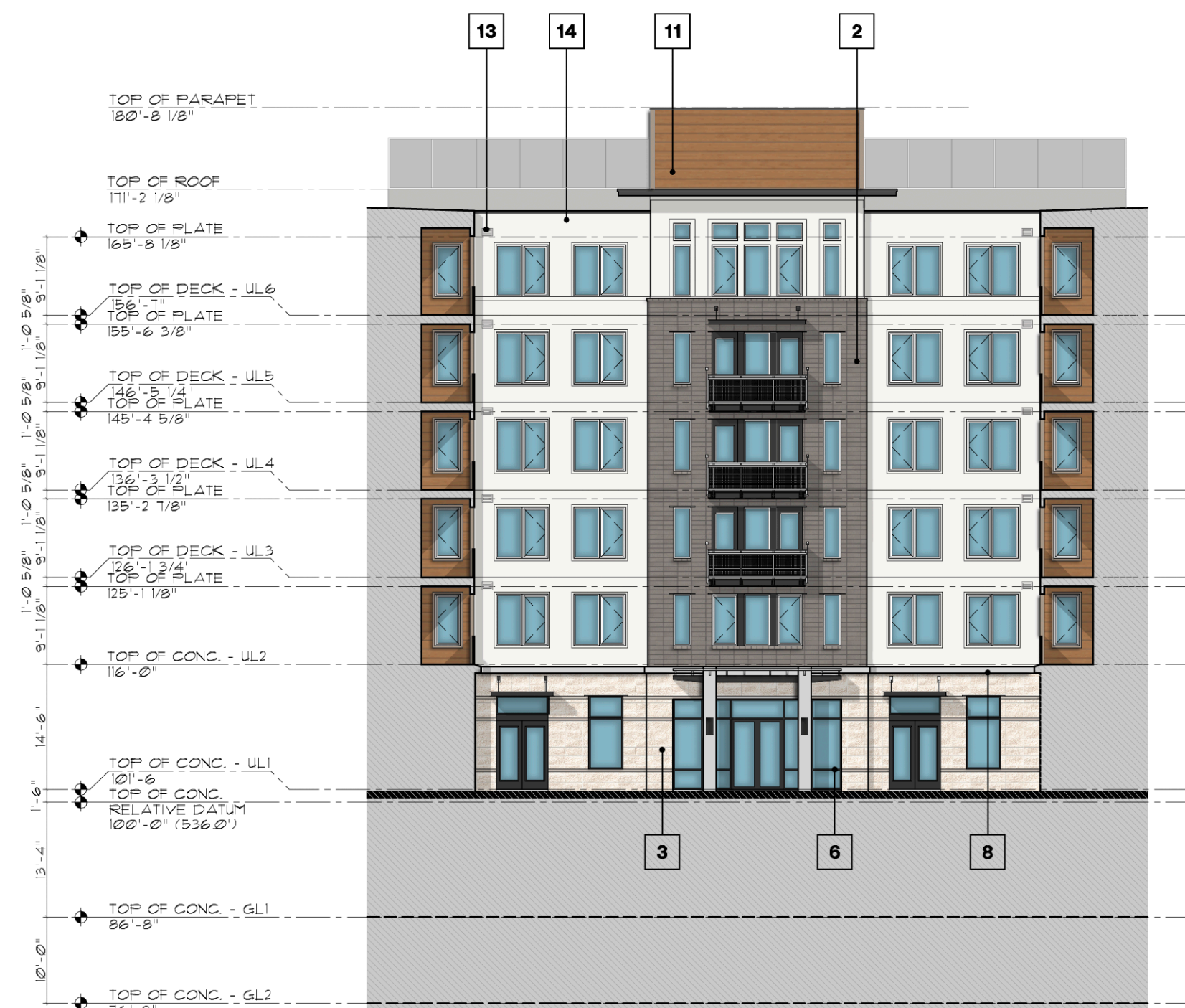
01 INTERIOR COURTYARD EAST ELEVATION SCALE: 1/16" = 1'-0"
