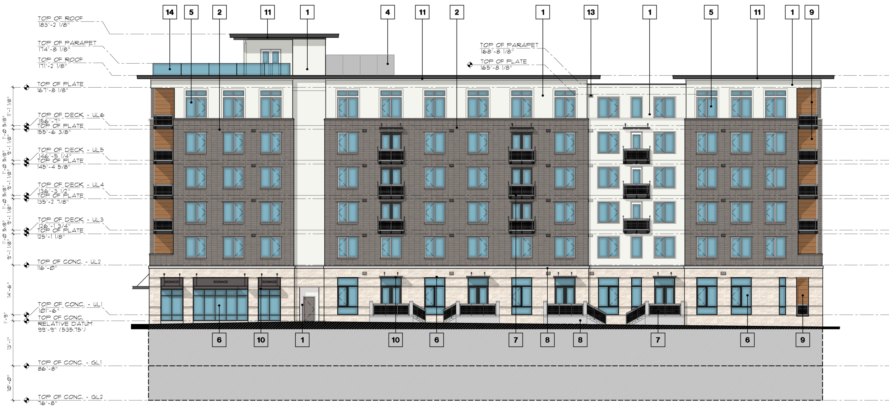
01 NORTH ELEVATION S.W. LANE SCALE: 1/16" = 1'-0"
