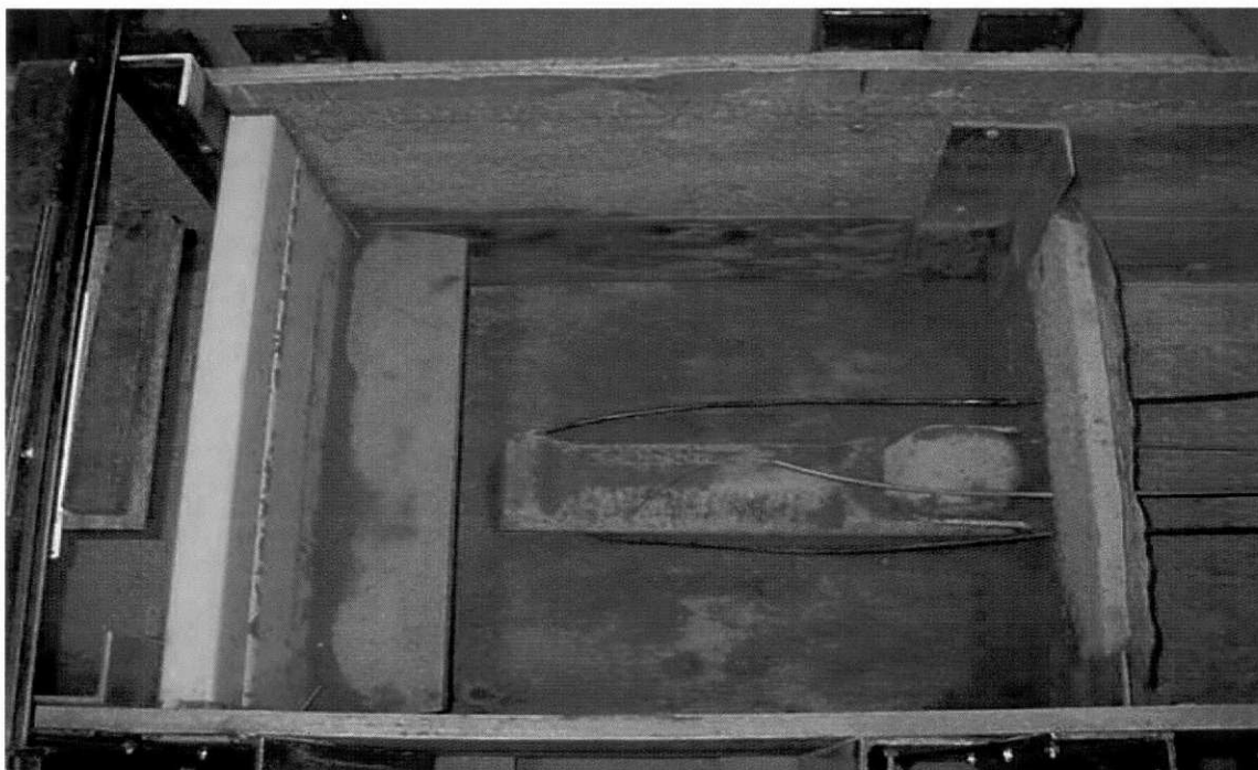
Figure 6: Orientation of Lock + Load retaining wall specimen (London counterfort) in soil pullout box showing tell-tale extensometers.
