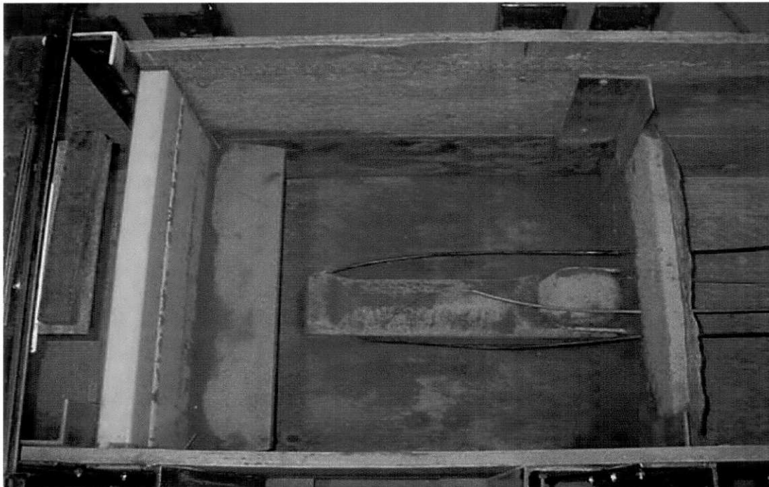
Figure 6: Orientation of Lock + Load retaining wall specimen (London counterfort) in soil pullout box showing tell-tale extensometers.
