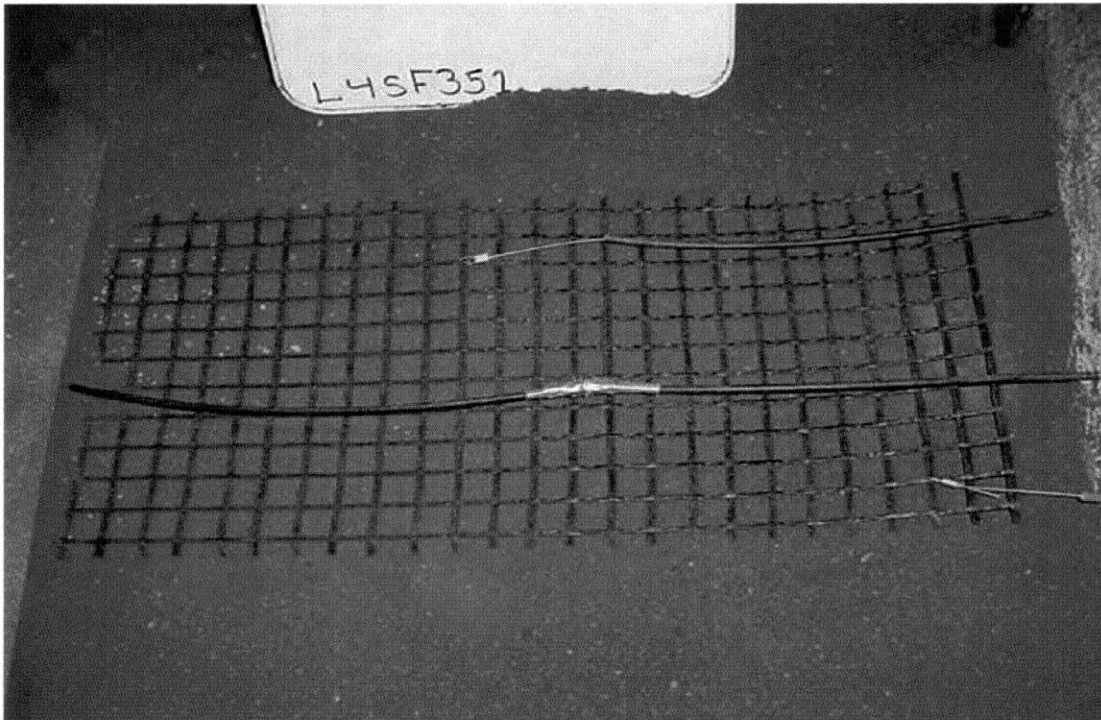
Figure 9: Exhumed Syntex SF35 geogrid specimen from Test 1 , after testing under a confining pressure of 5 kPa.
