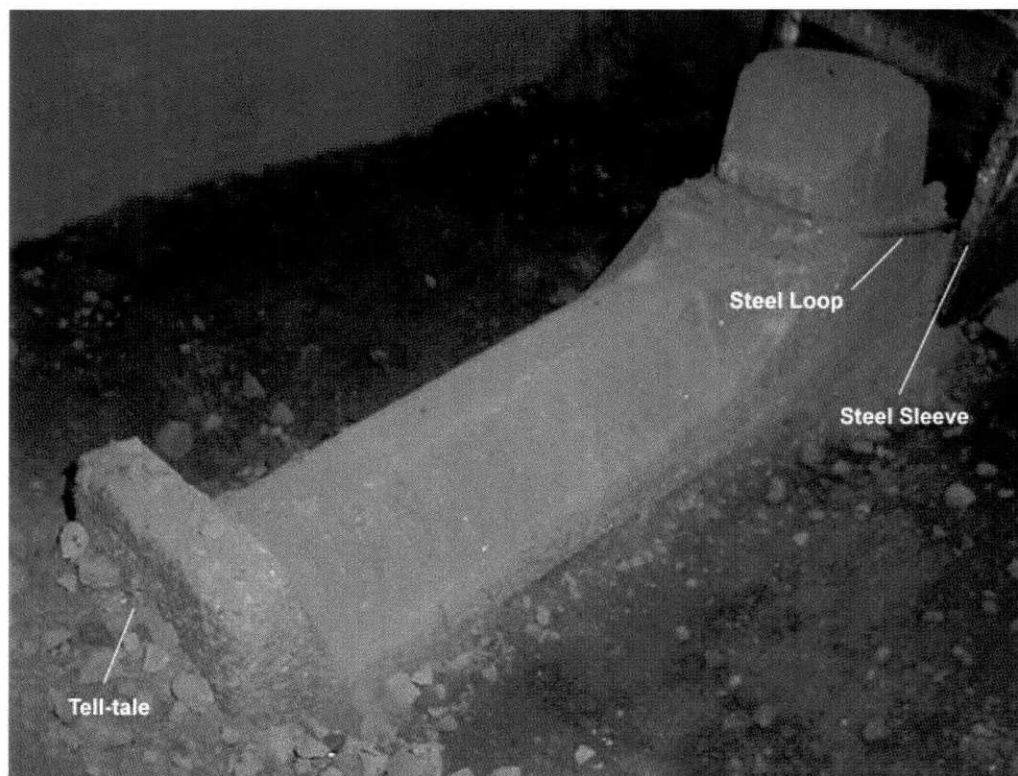
Figure 3: Photograph of a Lock+Load counterfort unit showing the general set-up in the soil pullout box.
