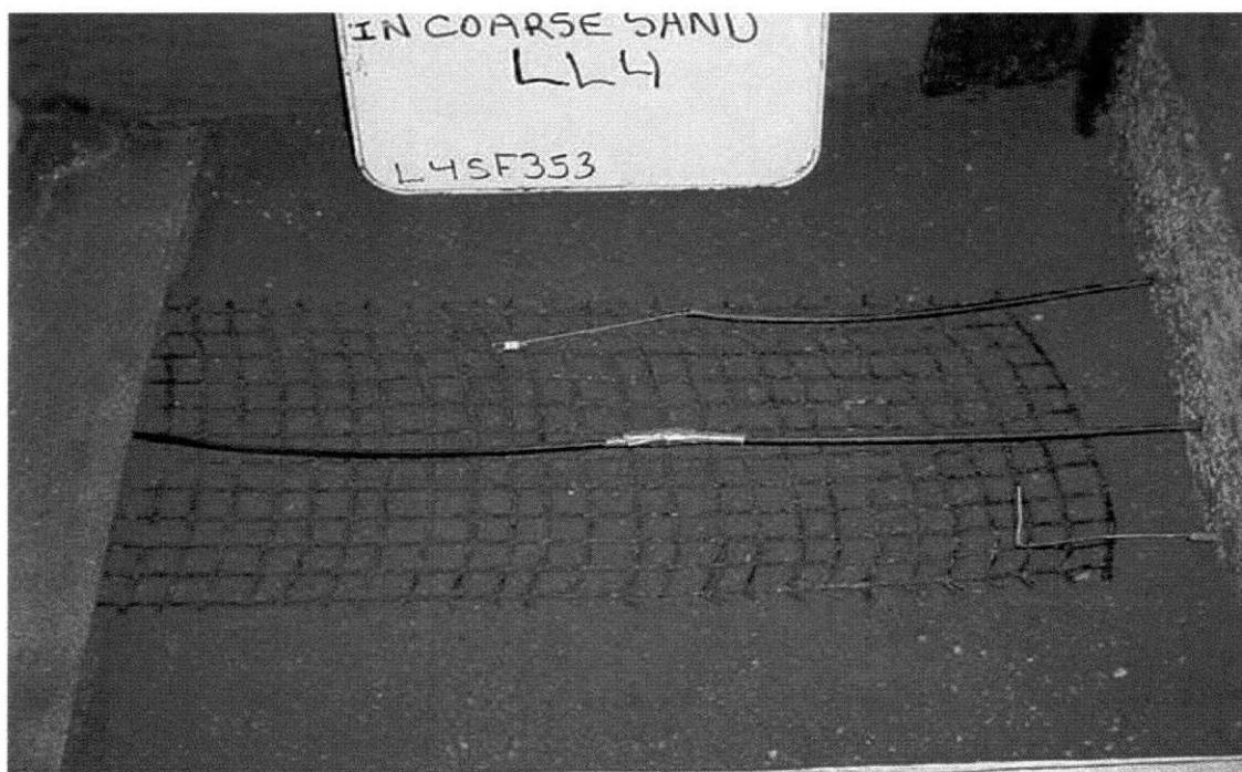
Figure 11: Exhumed Synteen SF35 geogrid specimen from Test 3 , after testing under a confining pressure of 18 kPa.
