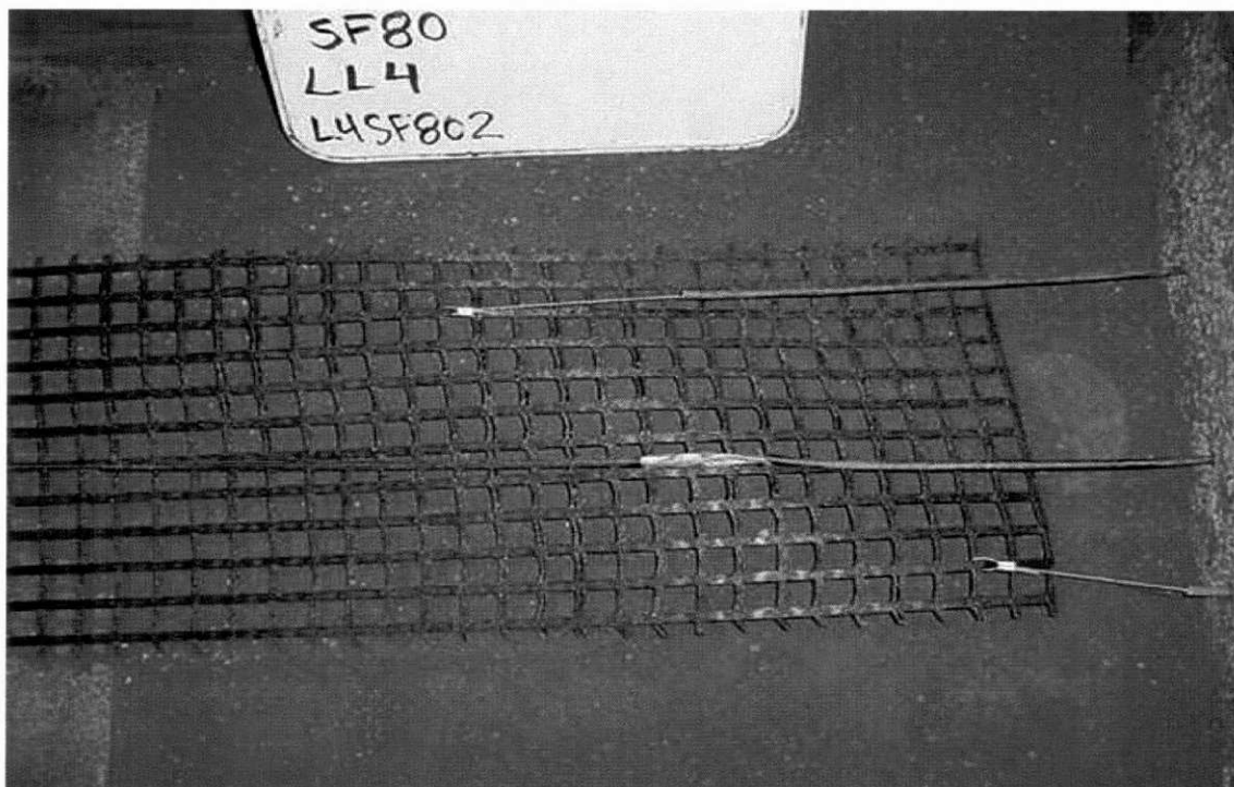
Figure 10: Exhumed SF80 geogrid specimen from Test 2 , after testing under a confining pressure of 18 kPa.
