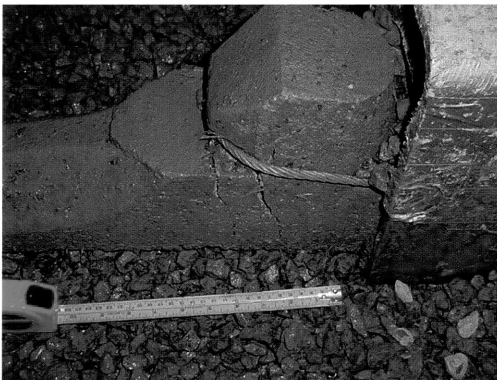
Figure 10: Photograph of exhumed specimen from Test 1 showing cracks of the counterfort head (confining pressure of 40 kPa).
