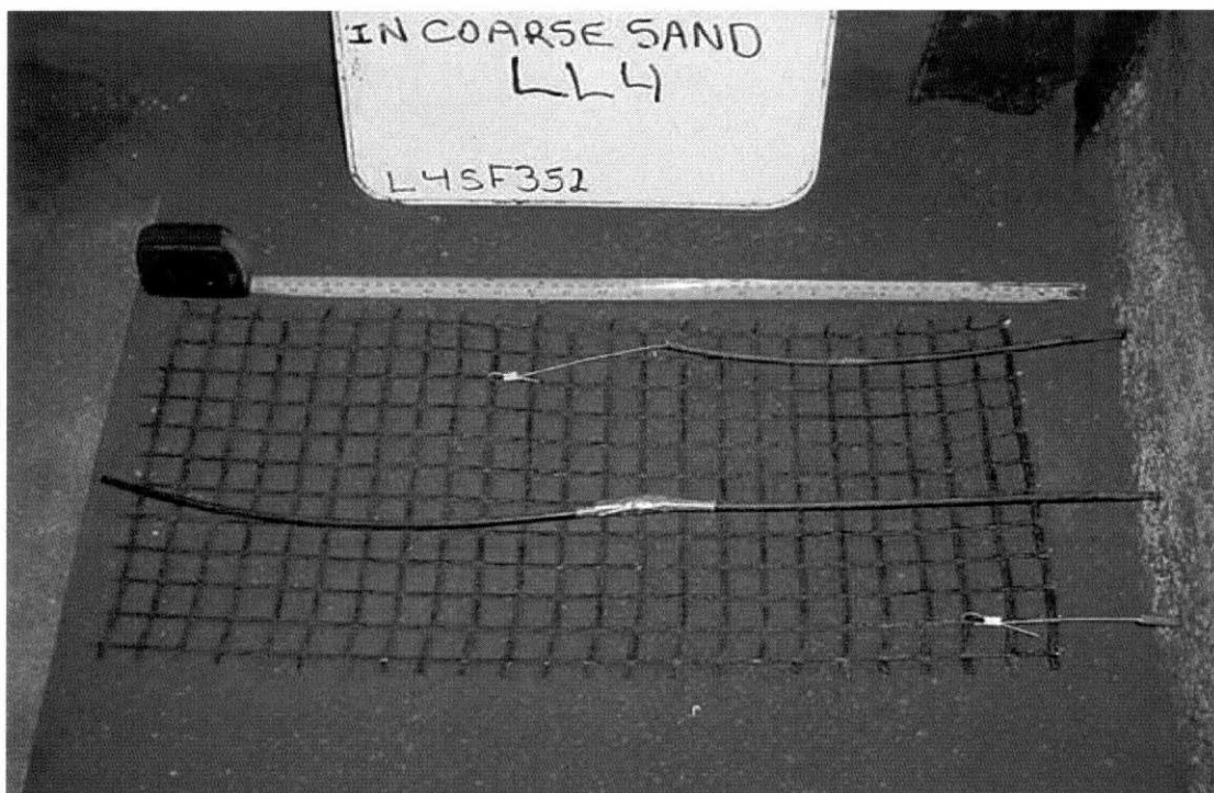
Figure 10: Exhumed SF35 geogrid specimen from Test 2 , after testing under a confining pressure of 12 kPa.
