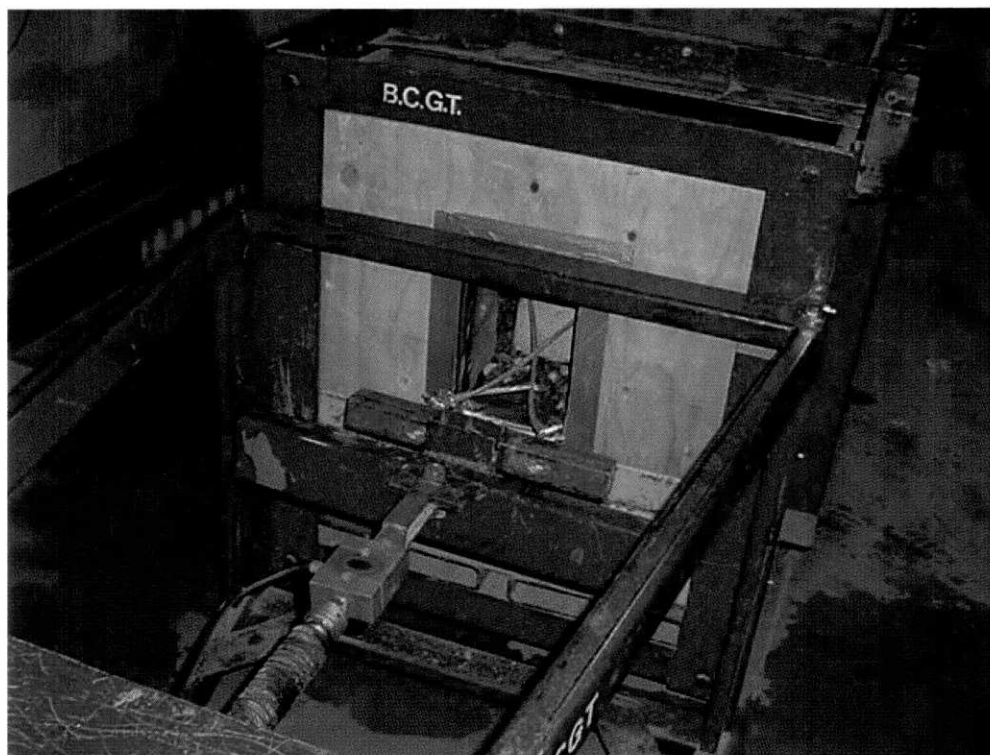
Figure 7: View of front wall panel and steel cable clamp arrangement at the front of pullout box.
