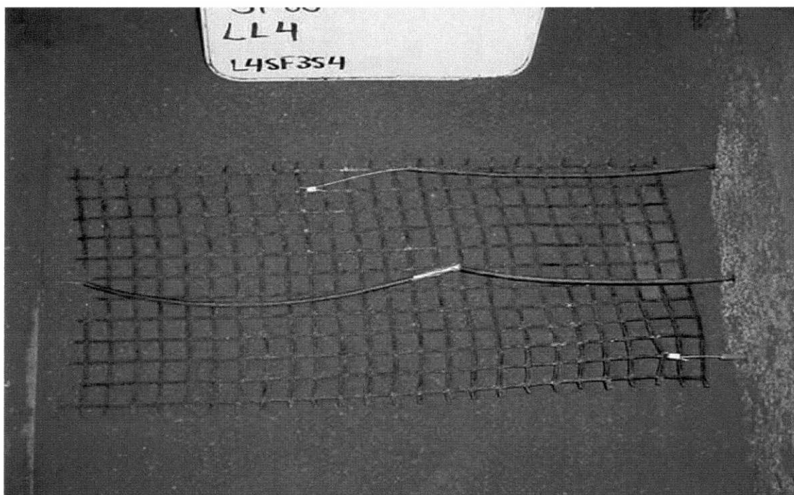
Figure 12: Exhumed SF35 geogrid specimen from Test 4 , after testing under a confining pressure of 25 kPa.
