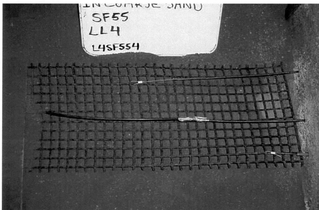
Figure 12: Exhumed SF55 geogrid specimen from Test 4 , after testing under a confining pressure of 32 kPa.
