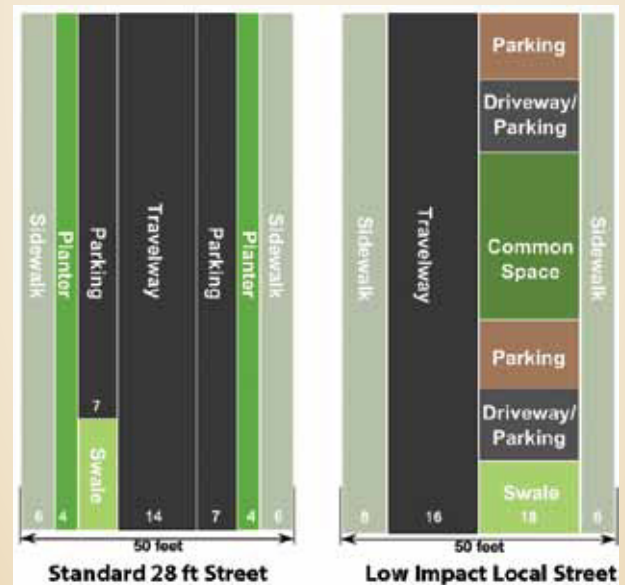
Figure 9: Diagram of low impact and standard streets
