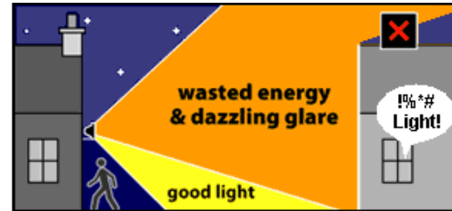
BADLY AIMED 500W HALOGEN FLOODLIGHT
