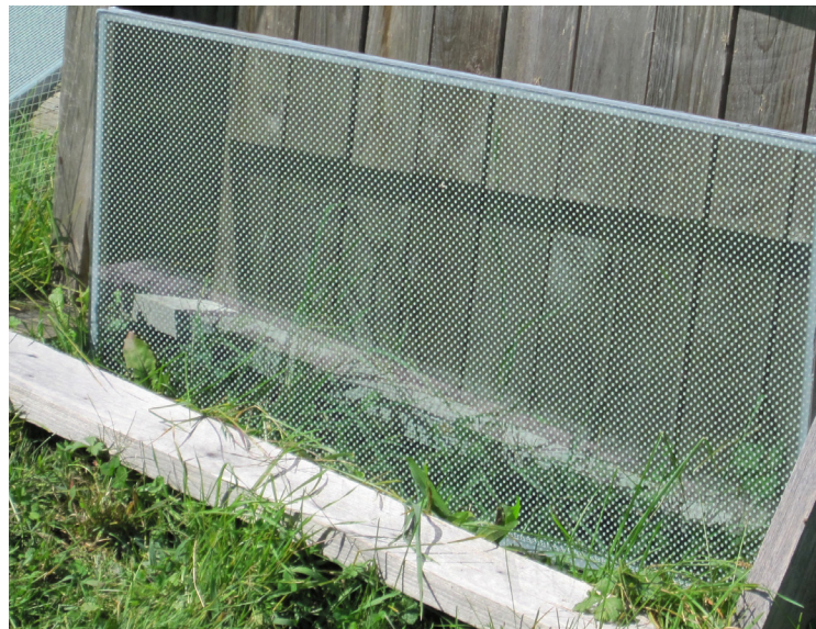
Patterns with more contrast and distinct spaces, such as the one shown on the left, are much more effective than repeating, all-over patterns like the one shown above. Photo: Christine Sheppard, ABC
