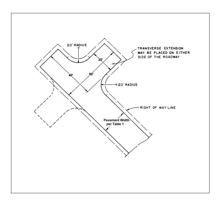
Figure 2 – Hammer Head Turnaround for Private Streets less than 300 feet Long
