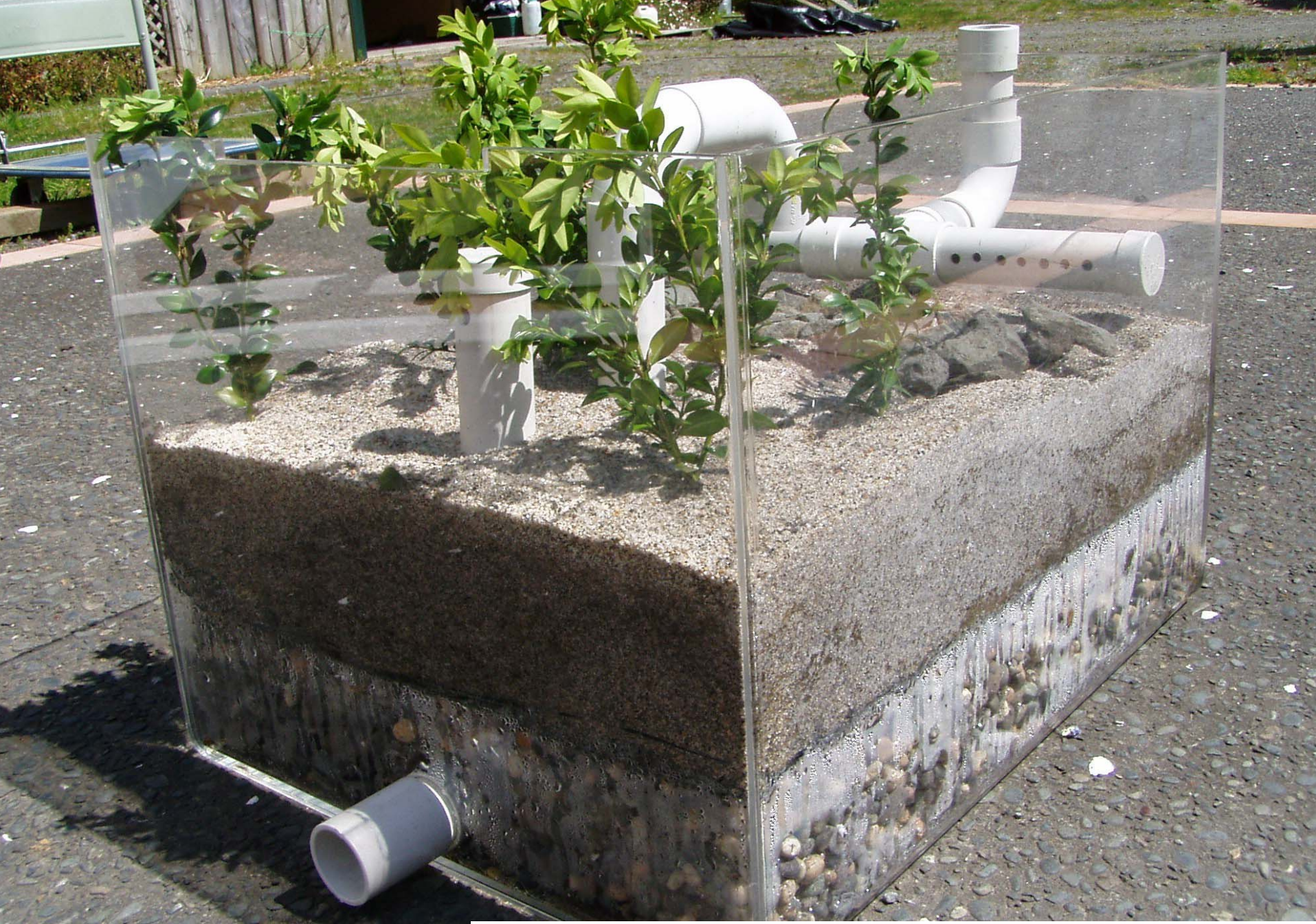
Flow-through planter test in New Zealand
