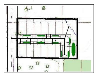
Step 3: Design pollution reduction and flow control facilities from Chapter 2.0: Stormwater Management Facility Design. Form SIM will be used to size the vegetated street swales to meet pollution reduction and flow control requirements. From this form, the sizing factor for vegetated swales is 0.09. The required square-footage of swales is: 19,000 square feet x 0.09 = 1,710 square feet. If the width of the swales is 7 feet, the required total length of swales is 244 feet.
