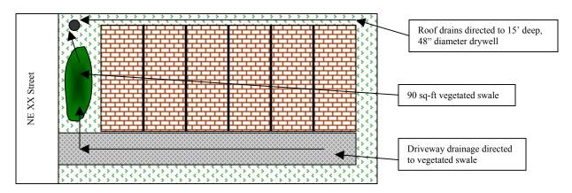
Soakage trenches used for rooftops and driveway, with a pollution reduction facility for the driveway:
