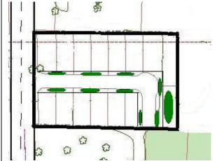
2) If there are sufficient areas on-site to use surface infiltration facilities to meet stormwater destination requirements, infiltration tests must be done to verify that the minimum rate of 2 inches per hour is met, and that the maximum drawdown time for all surface infiltration facilities will not exceed 30 hours.
