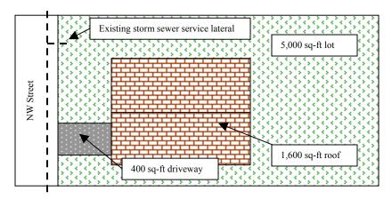
**Step 1**: Determine the stormwater disposal point for the site. Use **Exhibit 1-1**: **Stormwater Destination/Disposal Hierarchy** (in Chapter 1.0)
