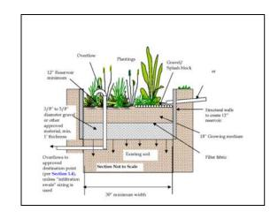
Form SIM will be used to size the infiltration planter to meet pollution reduction requirements. From this form, the sizing factor is 0.06. The required squarefootage of planter is: 5,000 square feet (parking lot area)  $\times 0.06 = 300$  square feet. The planter will be 3 feet wide by 100 feet long, and will include an overflow catch basin plumbed to an on-site drywell or soakage trench.
