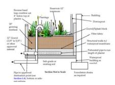
Step 3: Design pollution reduction and flow control facilities from Chapter 2.0: Stormwater Management Facility Design. Form SIM will be used to size the flow-through planters to meet pollution reduction and flow control requirements. From this form, the sizing factor for flow-through planters is 0.06. The required square-footage of planters is: 7,000 square feet (rooftops + driveway)  $\times 0.06 = 420$  square feet. The planter can be split up and
