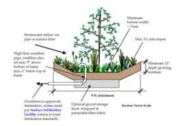
Form SIM will be used to size the vegetated swale to meet pollution reduction requirements. From this form, the sizing factor for vegetated swales is 0.09. The required square-footage of swale is: 1,000 square feet x  $0.09 = \underline{90}$  square feet. The swale will be 5 feet wide by 18 feet long, and will include an overflow catch basin plumbed to the site's drywell or soakage trench.
