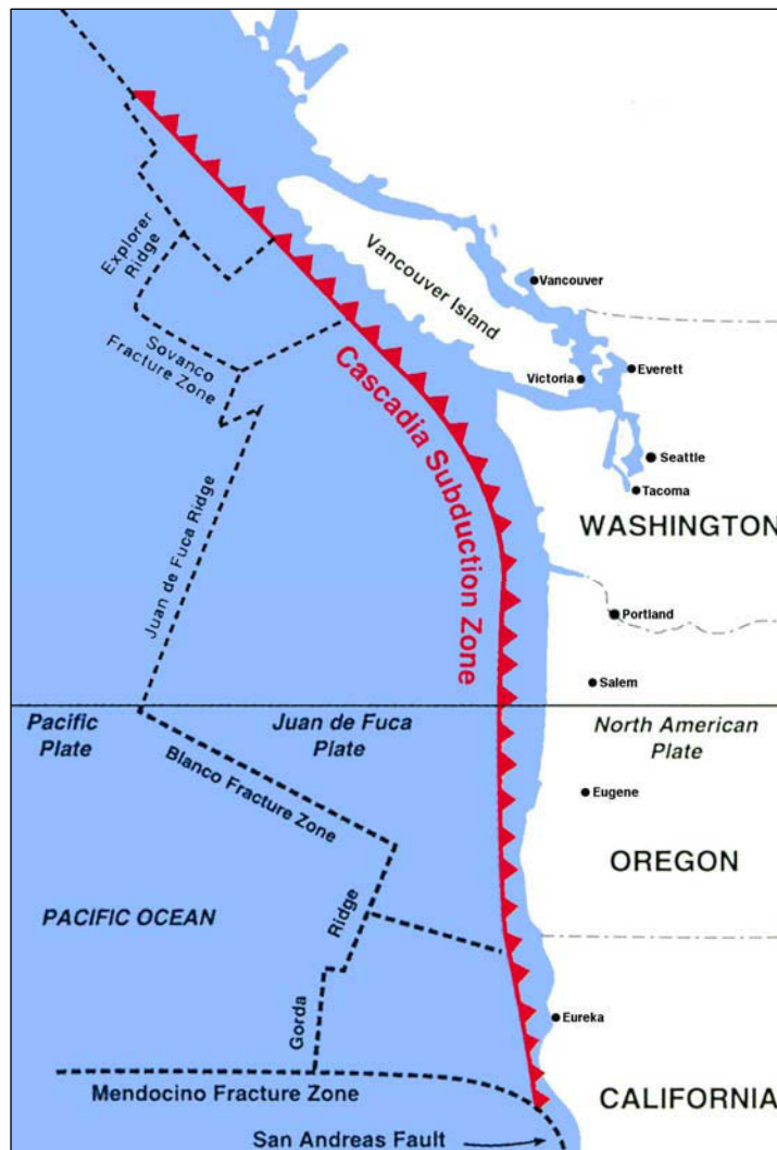
Figure J-B1a Earthquake Subzone Map
