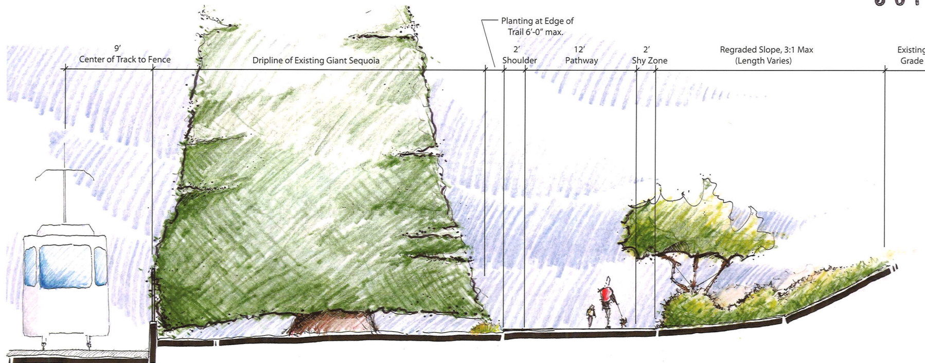
FIGURE 59: Project alignment and Trolley Trail cross section
