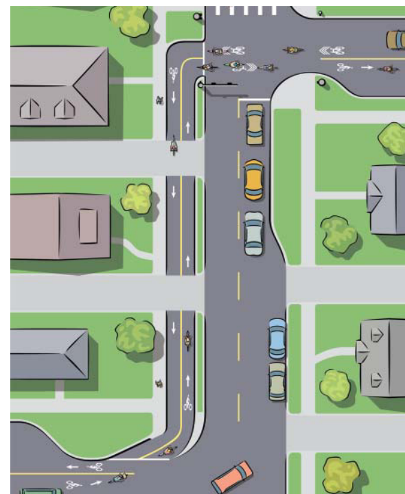
Concept of a bicycle boulevard crossing at an offset intersection with a two-way cycle track on the arterial street
