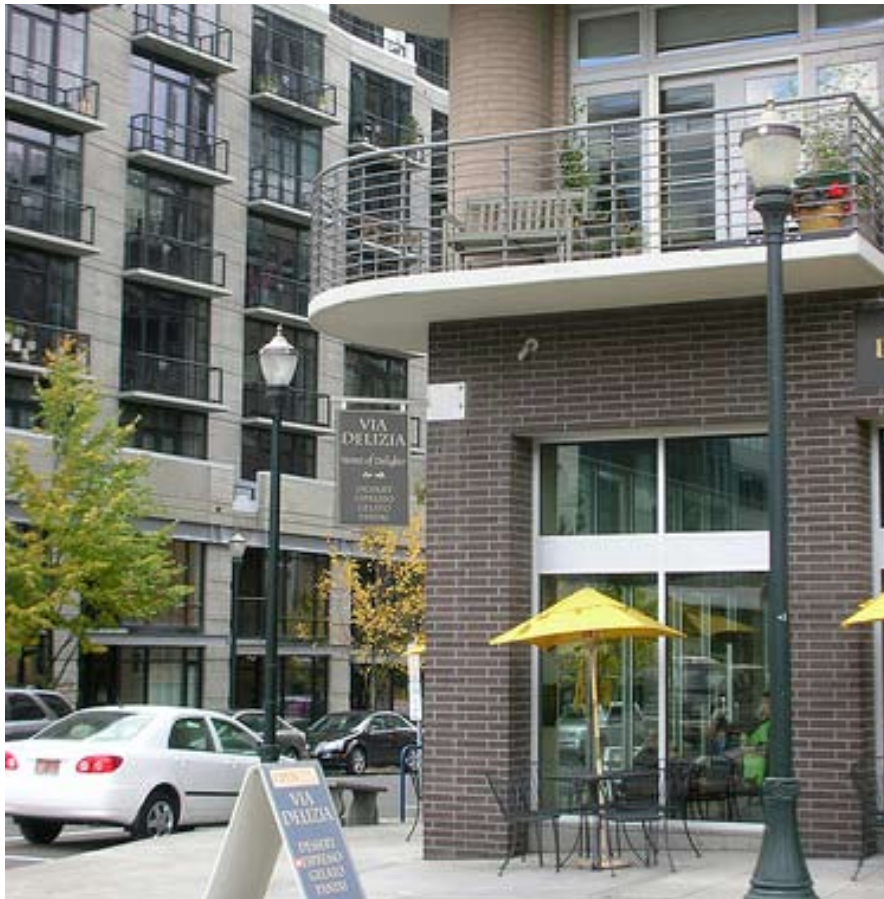
The Bridgeport Condominium Building on NW 11th creates a fine-grained pedestrian environment by providing outdoor seating and large windows to its ground floor retail. Tall ground floor ceiling heights as well as a differentiated brick color add prominence to the ground level. Residential balconies offer some weather protection and articulation.
