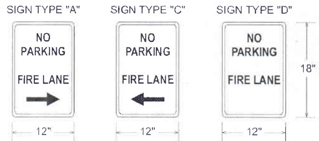
FIGURE D103.6 FIRE LANE SIGNS
