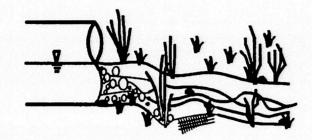
**Description:** In the past, streams were channelized and routed into pipes, combined with sewage, and discharged to the Willamette River. Later interceptors were built to collect dry weather flow and carry it to a treatment plant. Currently, stream inflow competes with other basin inflow for interceptor capacity. Removal of stream flow by diverting it to a new storm drain system or daylighting the stream would provide additional interceptor capacity for combined sewage.
