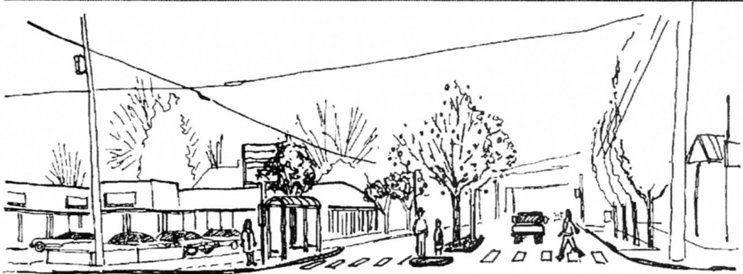
PROPOSED: Plan for improvements at 41st Avenue shows effect of a median refuge island and a transit curb extension.
