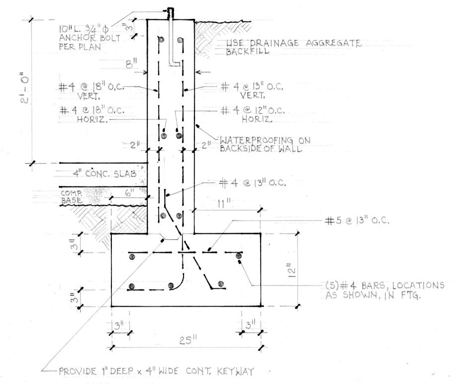
DETAIL - CONCRETE RETAINING WALL
