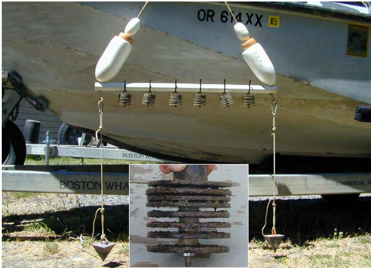
Figure 2. Hester-Dendy multiple-plate sampler (inset) and array used for epibenthic invertebrate surveys of the lower Willamette River, May-June 2003.
