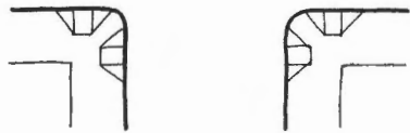
Curb ramps are located at each end of each crosswalk at a “T”
