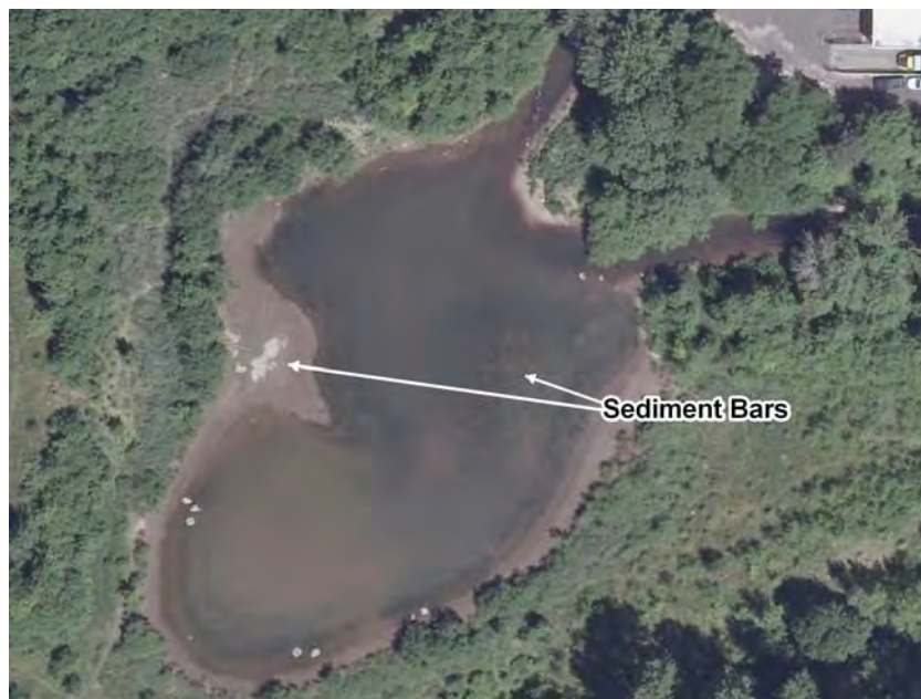
Photo 17: Sediment bars forming in Brookside embayment pond, 2008 aerial.
