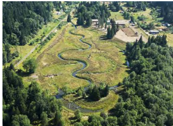
Photo 21b: The Schweitzer Natural Area. Johnson Creek now meanders through the site mimicking a more natural system. Backwater channels provide high-flow refuge.
