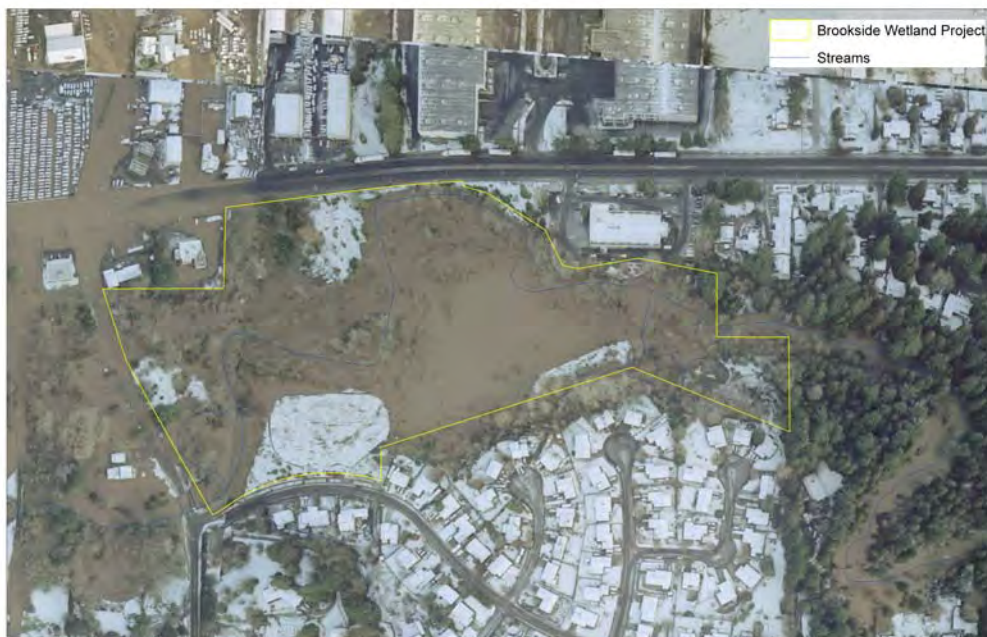
Photo 16: Brookside Wetland during the peak of the January 2009 flood which filled the project to capacity.
