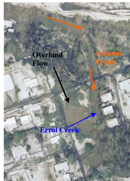
Photo 11: Aerial of January 2009 flood. Johnson Creek accesses flood storage at Errol Confluence via backwater and overland flow.
