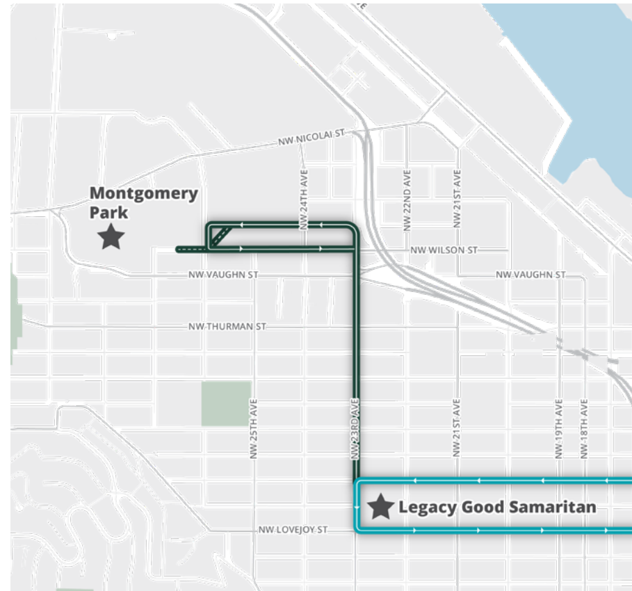
The preferred alignment is a direct route to Montgomery Park, extending via a two-way on NW 23rd Avenue to a new parallel one-way couplet along rebuilt and extended NW Wilson and NW Roosevelt streets.
