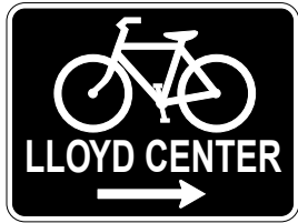
FIGURE A4.19 Directional Bicycle Route Sign
