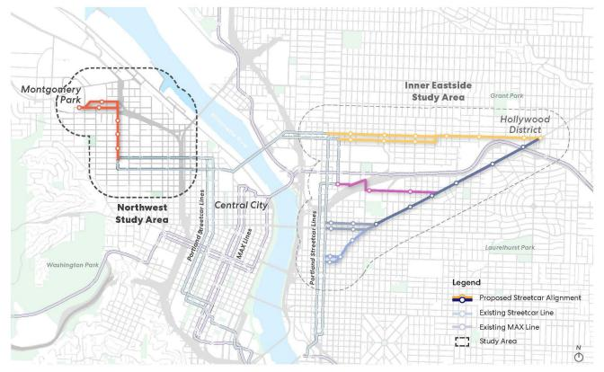
Potential westside and eastside alignment options studied as part the MP2H process could expand the streetcar system.
