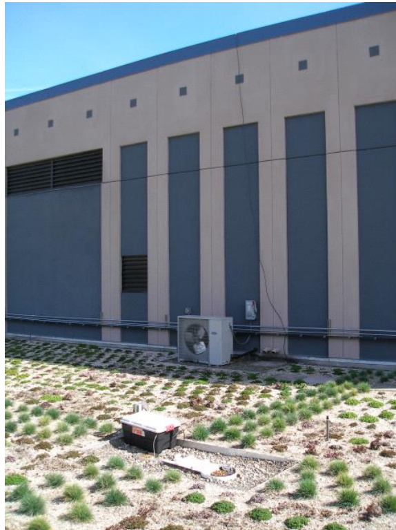
Figure PB-1: Portland Building Ecoroof (SW corner) – monitoring setup (flume, data logger, & raingage)
