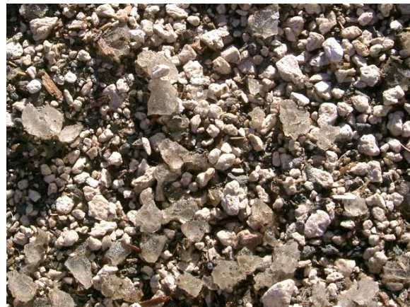
Figure PB-9: Ecoroof cross-section (left) and Stockosorb® gel in the soil media (right)
