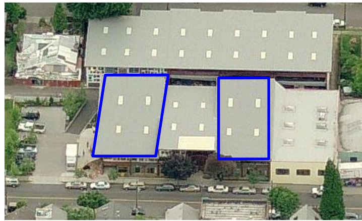
Figure RC-3: Roof area draining to planters
