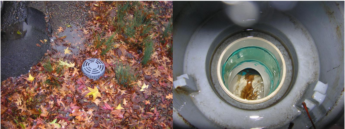
Figure OZ-10 – overflow sampling location (Row 7); flow in underdrain (right) is pumped into a sample container through the overflow dome
