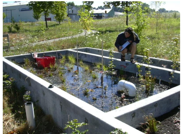
Figure 3-1: Recording drawdown rates at the WPCL Test Planters
