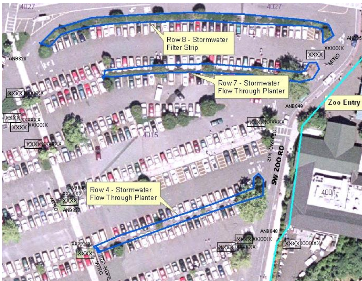
Figure OZ-1 – Facility Overview
