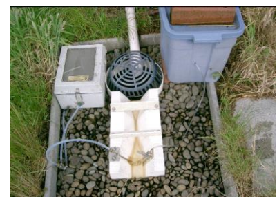
Figure HA-2: Monitoring setup – flume and datalogger
