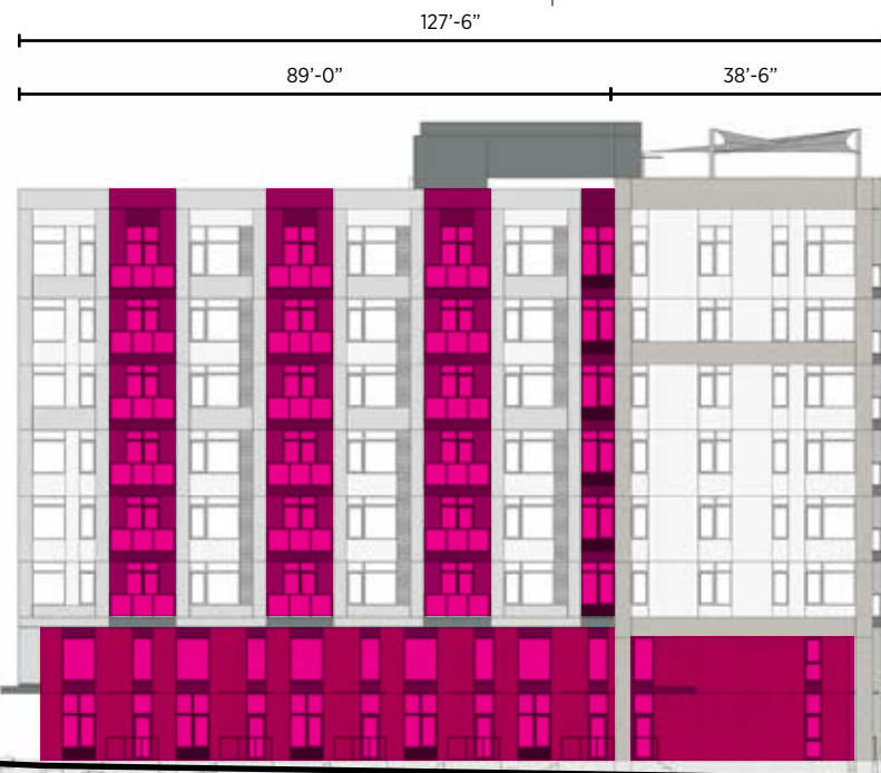
NORTH (NE PACIFIC ST.) *NOT A PUBLIC RIGHT OF WAY HIGHLIGHTED AREA _ SETBACK GREATER THAN 2FT = 40%
