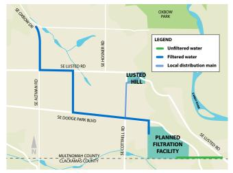
**Purpose:** Connects the water filtration facility to the existing Bull Run water system and improves resilience by allowing an aging segment of pipeline to be retired.
