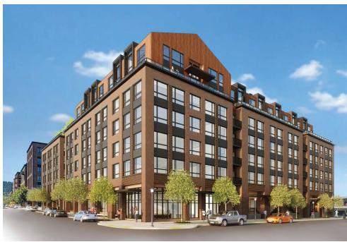
3. Gable-end form adjacency to lower parapet at SE, NE and NW corners of building is visually and functionally awkward due to the unusual scale and location of the element. The 'scoop dormers' are more successful;
