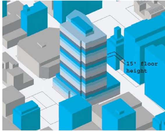
(b) each polygon is divided into floors; each floor's square footage can then be calculated
