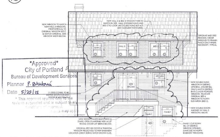
PROPOSED EAST / REAR EXTERIOR ELEVATION
