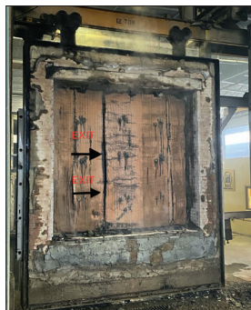
**After Hose-Stream Test
