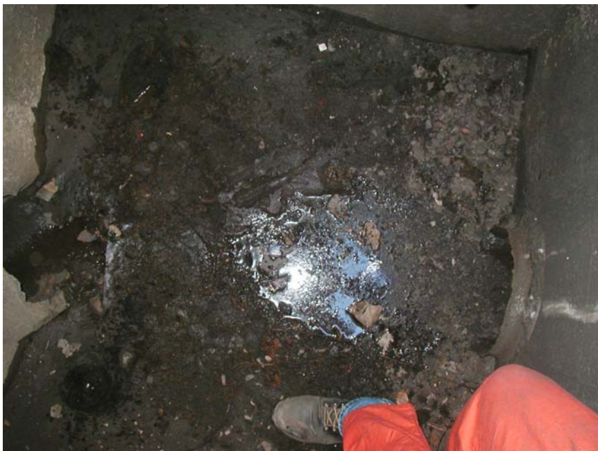
Photo 7 (July 2006). Catch basin ANE475, with an inlet from Cascade General and an outlet to Basin S-6. Solids were collected using a stainless steel spoon and bowl.
