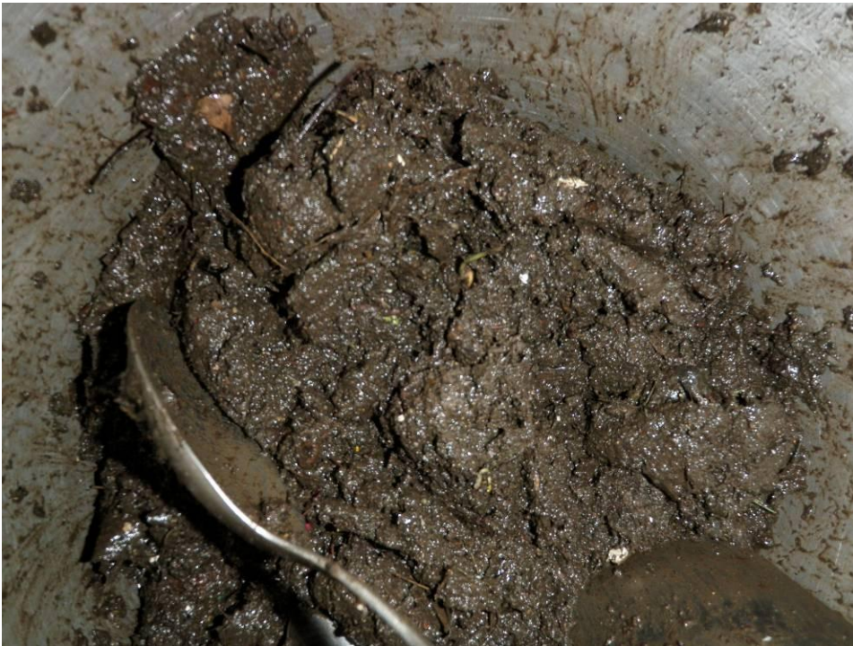
Photo 16 (September 7, 2010). Final homogenized composite sample (N. Lombard-1) from N. Lombard St. catch basins (ANF066, ANF067, ANF069, ANF072, ANF074, ANJ736) within Basin 52C.
