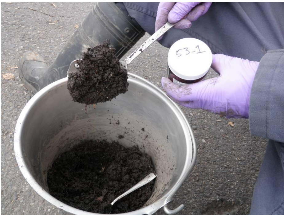
Photo 27 (September 8, 2010). Final homogenized composite sample (N. Lombard-3) from catch basins (ANF032, ANF036, ANF037, ANF041, ANF042) within Basin 53.
