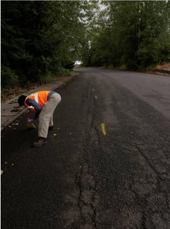
Photo 3 (September 7, 2010). Sweeping of sediments from cracks and depressions on N. Sever Rd. at subsample area 2.
