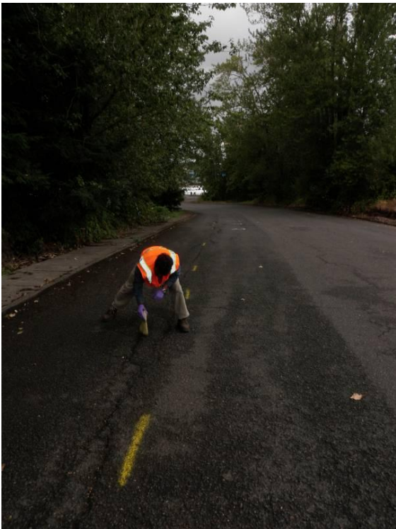
Photo 4 (September 7, 2010). Sweeping of sediments from cracks and depressions on N. Sever Rd. at subsample area 3.
