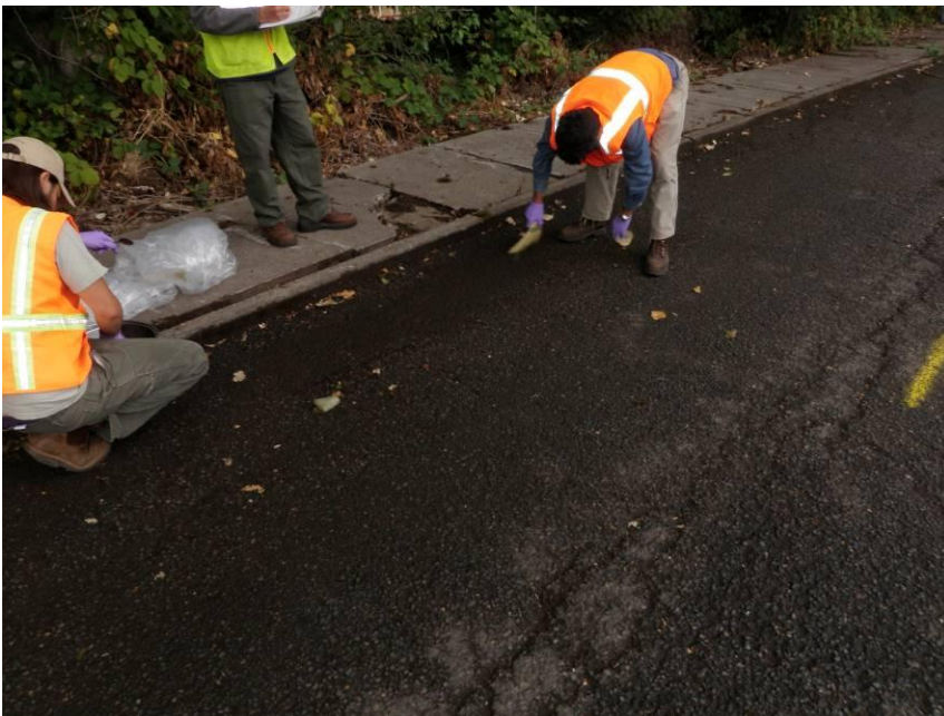
Photo 2 (September 7, 2010). Sweeping of sediments along N. Sever Rd. at subsample area 1.
