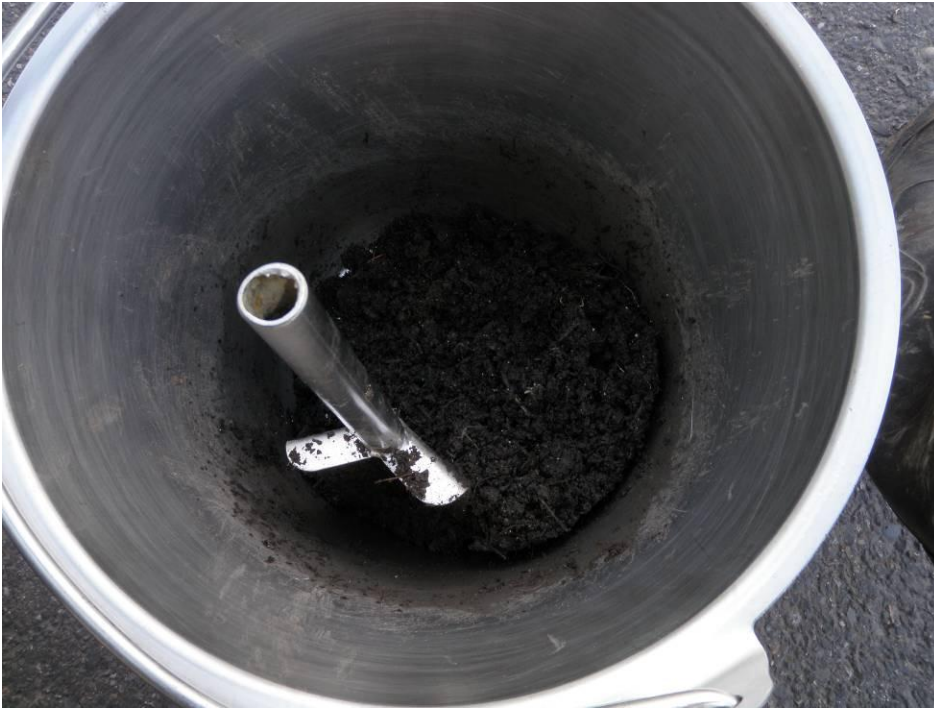
Photo 21 (September 8, 2010). Final homogenized composite sample (N. Lombard-2) from catch basins (ANK382, ANK385, ANK394, ANK400) between Basin 52C and Basin 53.
