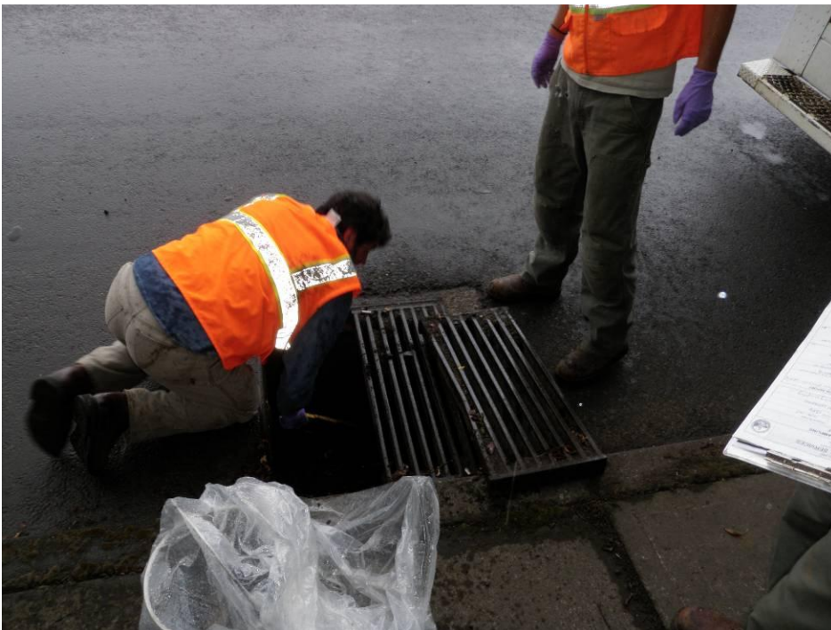
Photo 14 (September 7, 2010). Sampling of catch basin ANF072 for Basin 52C catch basin composite sample (N. Lombard-1).
