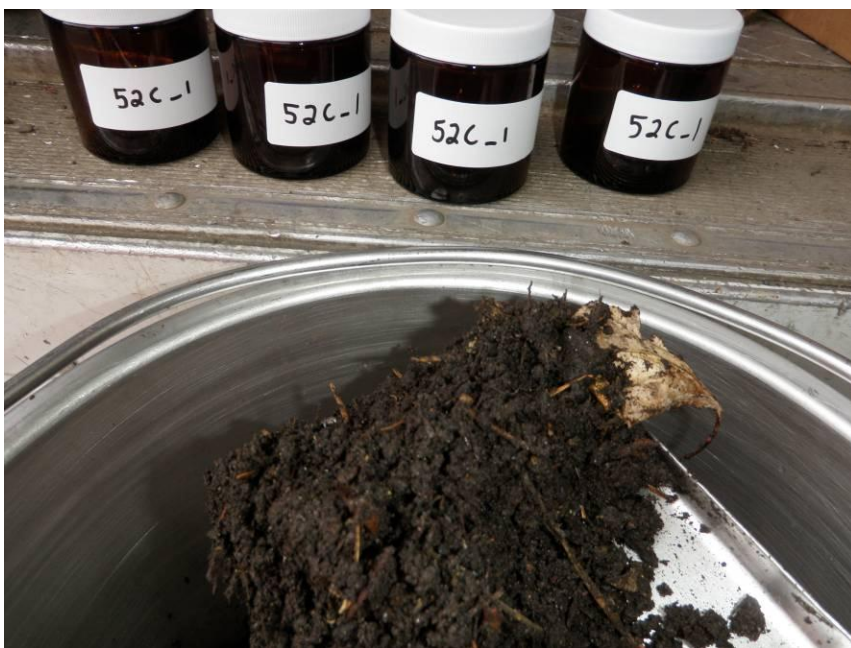
Photo 6 (September 7, 2010). Final homogenized composite sweepings sample (comprised of sub-samples areas 1-4) from N. Sever Rd. near intersection with N. Burgard Rd.
