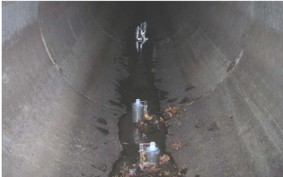
Photo 3 (October 2008). Two sets of installed sediment traps at sampling location ST1 (Manhole ABC311). The trap in the foreground is the farthest upstream.
