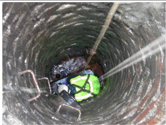
**Photo 5 (April 1, 2009).** Sampling flow from lateral entering Manhole ABC355 from the north (44\_SW3).
