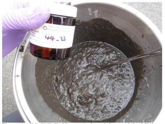
Photo 66 (April 28, 2010). Final homogenized sample from manhole ABC343.
