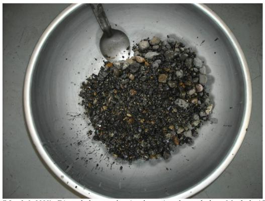
Photo 20 (March 9, 2009). Discarded coarse fraction from sieved sample from Manhole ABC278
