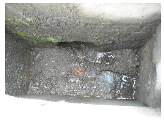
**Photo 54 (January 28, 2010).** Solids inside Catch Basin APG314, sampled and composited with solids from on top of filter fabric (preceding picture).
