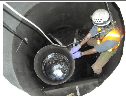
**Photo 41 (April 8, 2009).** Accessing Manhole AMQ287 (sedimentation manhole in N. Loring Street) for sampling.
