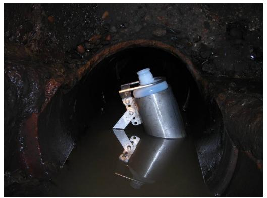
**Photo 17 (November 17, 2008).** Deployed sediment trap at sampling location ST1 (Manhole ABC352)
