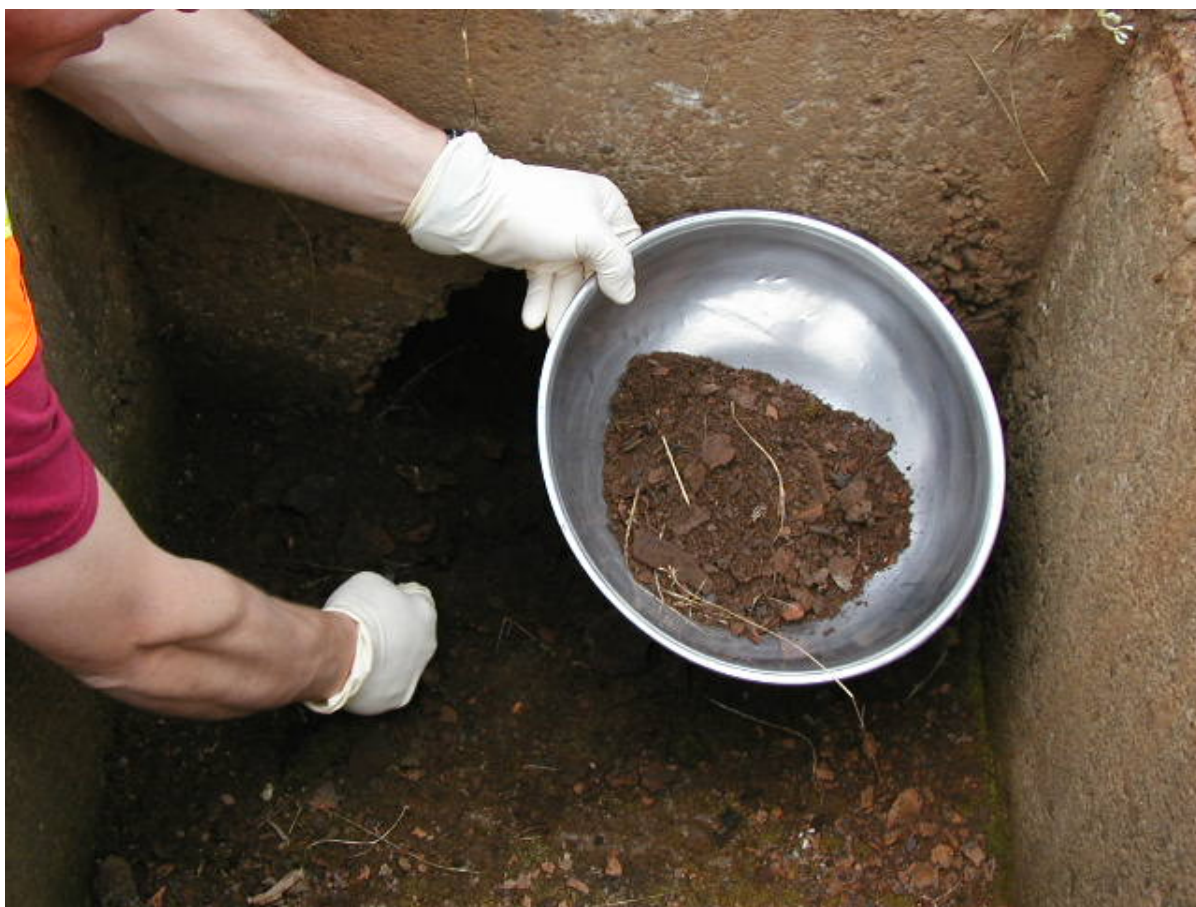
Photo 2 (June 2005). Sampling catch basin AMW708 with a stainless steel spoon and bowl.
