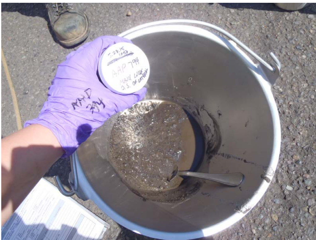
Photo 22 (May 28, 2015). Manhole AAP794. Inline solids sample collected from 48" main line downstream of manhole and Phillips #3 connection.
