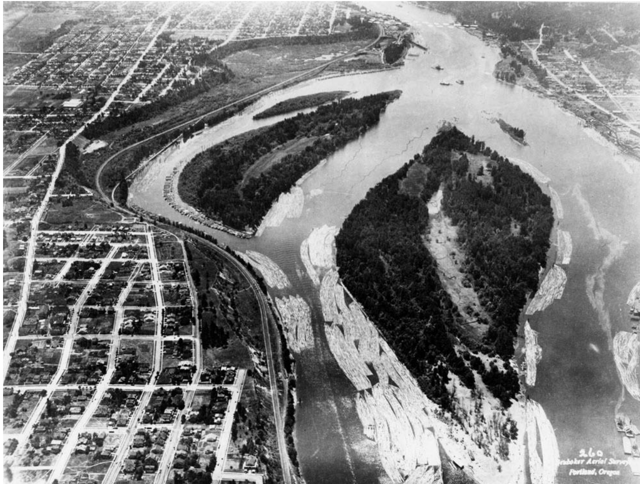
Figure 33: An historical aerial photo from 1926 showing Oaks Bottom and Ross Island. Consistent with the bank survey, the banks adjacent to the southern tip of Ross Island are low-lying, and the wetland appears to be hydrologically connected to the mainstem, whereas the banks further north along Holgate channel appear steeper.
