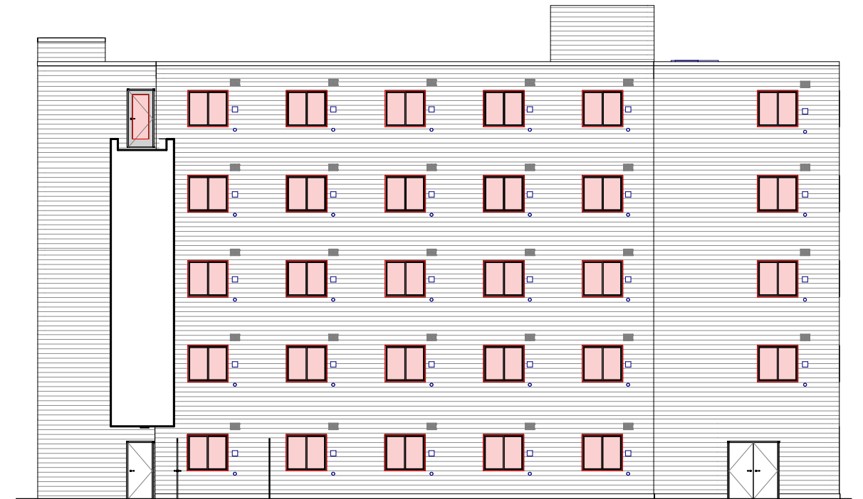
East Elevation A 13% glazing
