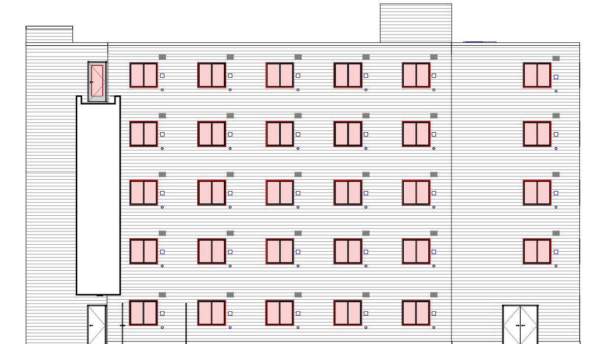
East Elevation A 13% glazing
