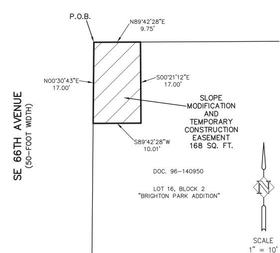
SLOPE MODIFICATION AND TEMPORARY CONST. EASEMENT R/W# 9404-21 PROJ# 1363
