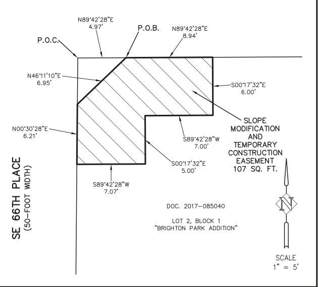
R/W# 9404-24 SLOPE MODIFICATION AND TEMPORARY CONST. EASEMENT PREPARED BY: MPS
