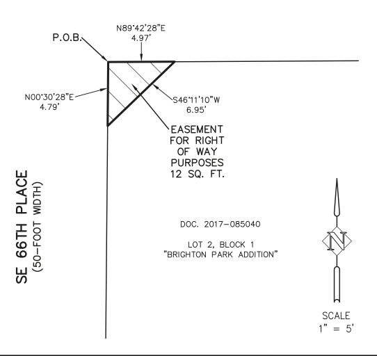
R/W# 9404-24 EASEMENT FOR RIGHT OF WAY PURPOSES PREPARED BY:MPS
