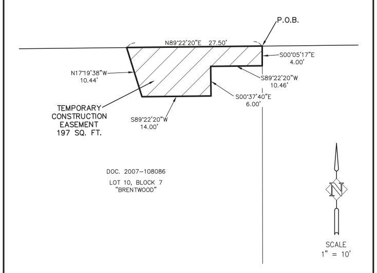
R/W# 9404-78 TEMPORARY CONSTRUCTION EASEMENT PREPARED BY: MPS
