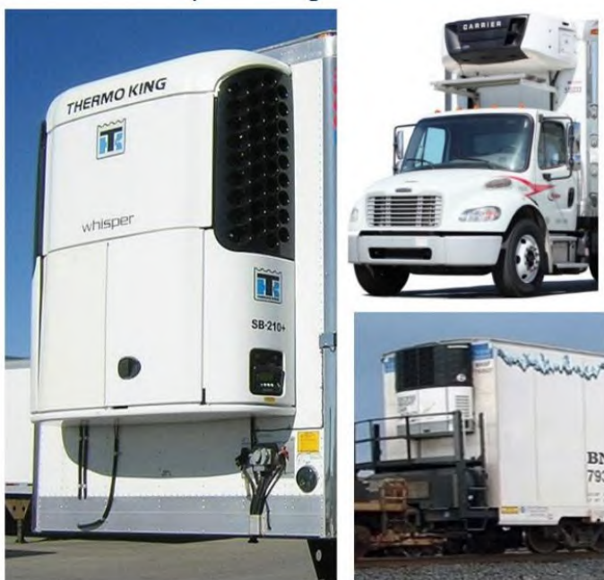
Figure 11: TRUs on Trucks, Trailers, and Rail Cars 42
