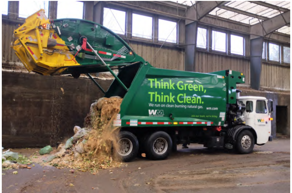
Above, a CNG-powered truck delivers commercial food waste to the North Portland transfer station. The waste will go to JC Biomethane to be digested and converted into electricity and soil amendments. Eventually, the hope is to collect the methane from the anaerobic digester and then turn that methane into renewable natural gas that can fuel trucks currently using CNG.
