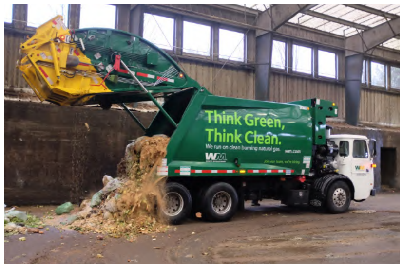
Medium- or heavy-duty trucks, like this Waste Management fleet truck, can run on CNG.
