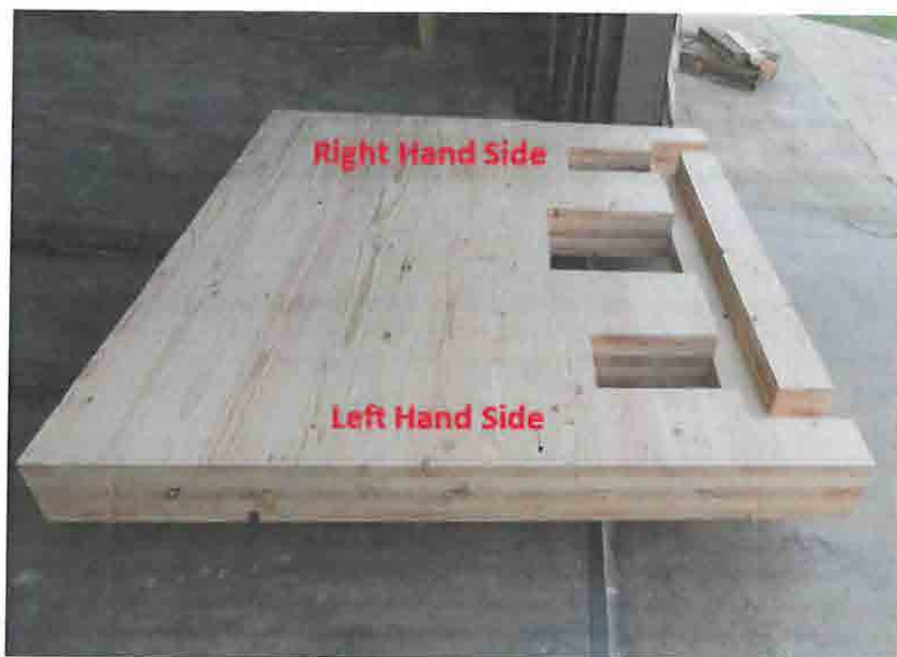
Figure B-1. CLT Panel Orientation for Thermocouple Installation.
