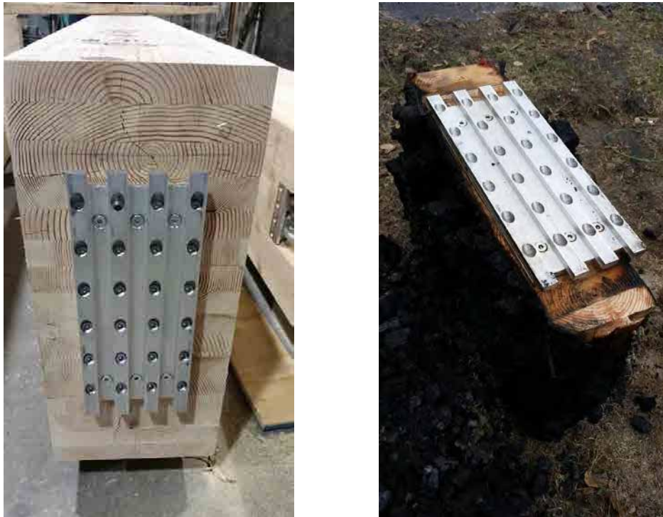
Figure 12 – Test 3 connector before and after test (beam cut for inspection after test)
