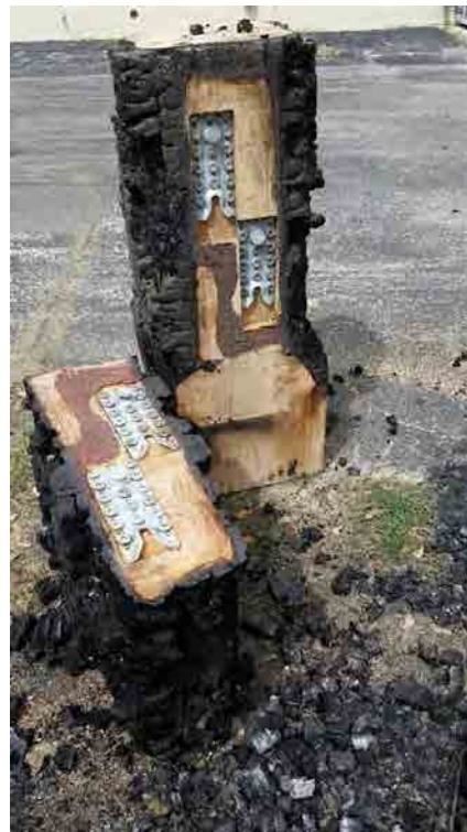
Figure 11 – Test 2 during test and post-test (beam and columns cut for inspection)
