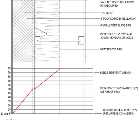
TYPICAL VAULTED ROOF ASSEMBLY - DEW POINT ANALYSIS
