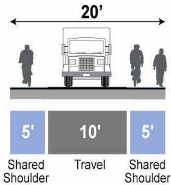
**Figure 3 - Shared roadway cross section**
