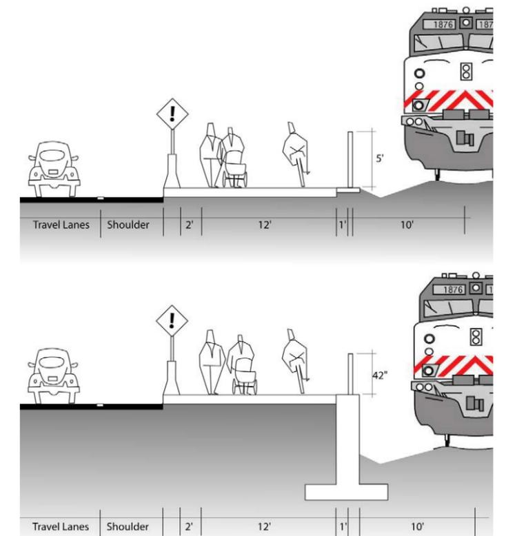
Typical cross-sections for a barrier-protected multi-use trail between travel lanes and rail line.
