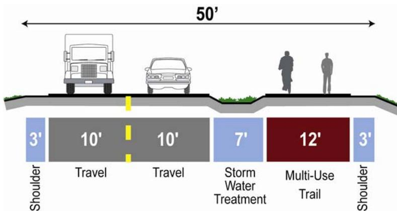
**Figure 1 - Roadway plus multi-use trail cross section**
