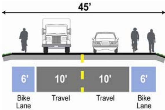
**Figure 2 - Roadway plus bike lanes cross section**
