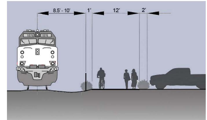
*Typical cross-section at rail-with-trail. Setback varies with track curvature.*
