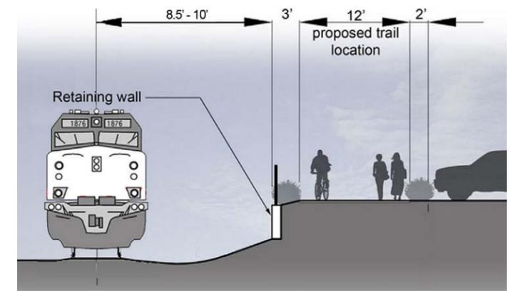
Rail-with-trail typical cross-section where trail is above rail. (Minimum distance center of track to fixed objects is 8.5', increases with curvature of rail alignment).
