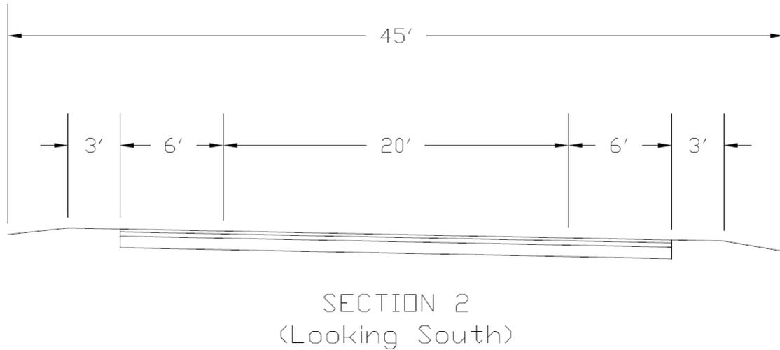
**Figure 2 – Roadway plus bike lanes cross section**
