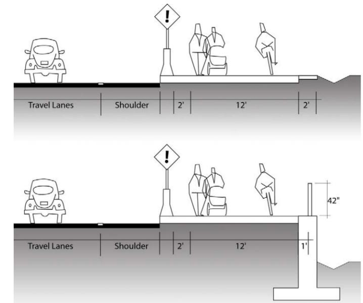
A barrier protected multi-use trail can be on-grade with the roadway, or supported by a retaining wall where the ground slopes away from the shoulder.
