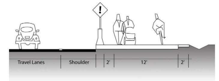
Typical cross-section for barrier-protected multi-use trail.
