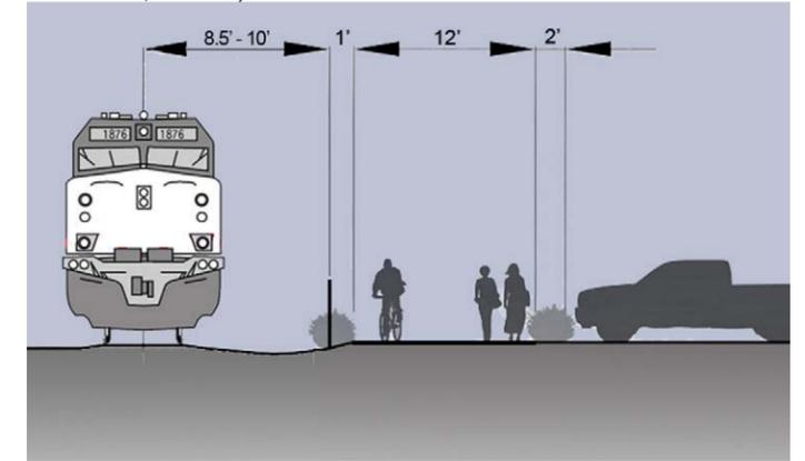
*Rail-with-trail typical cross-section. (Minimum distance center of track to fixed objects is 8.5', increases with curvature of rail alignment).*
