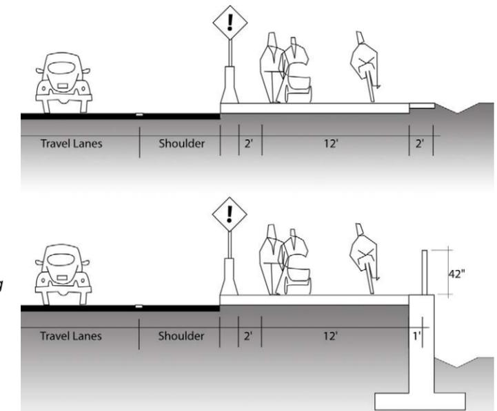
A barrier-protected multi-use trail will require modification of the roadway and could require retaining walls and/or changes to other improvements in and adjacent to the St Helens Road right-of-way.
