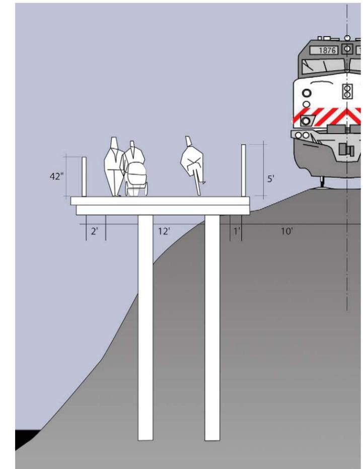
*A boardwalk structure could be built to traverse the narrow right-of-way overlooking the Willamette River.*
