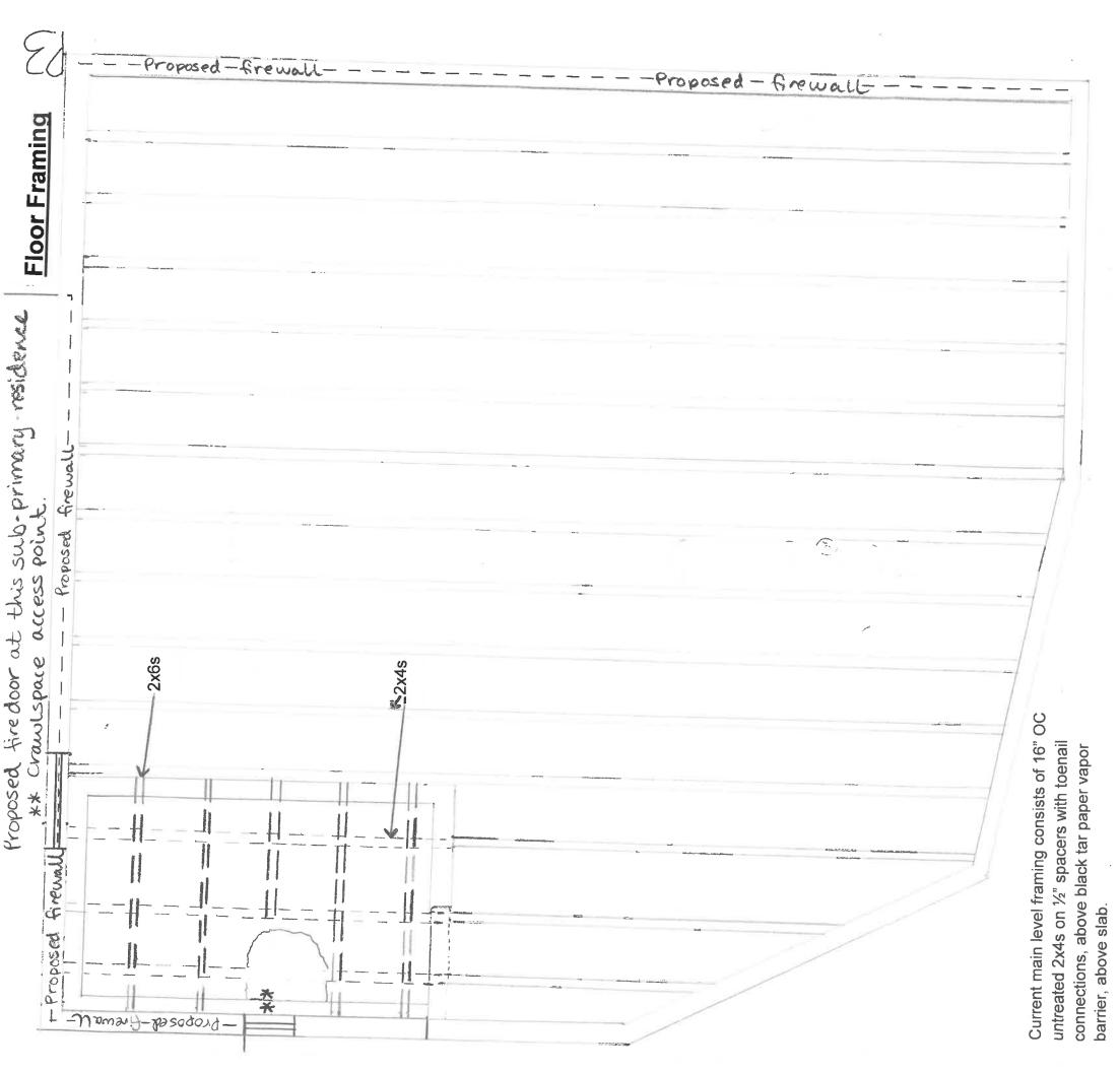
Propose to lift floor higher, for increased volume of vapor barrier atop existing concrete slab.
