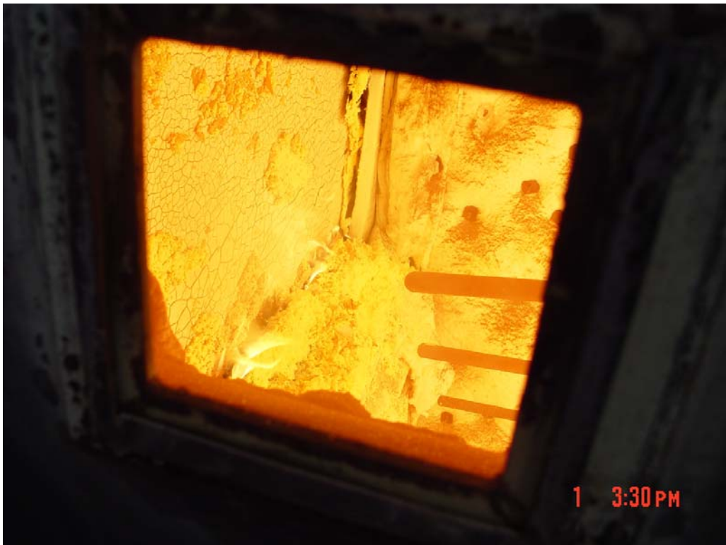
Photograph 6: Little intumescent remains and flames at bottom of sample near end of test
