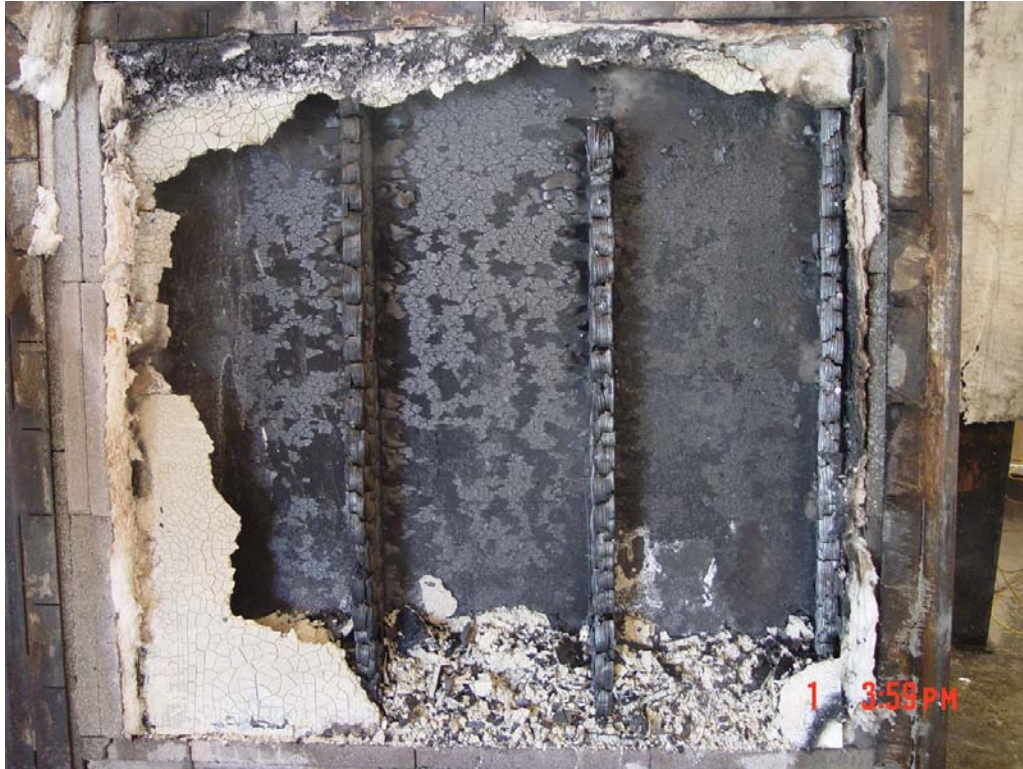
Photograph 9: Exposed sample face post-test
