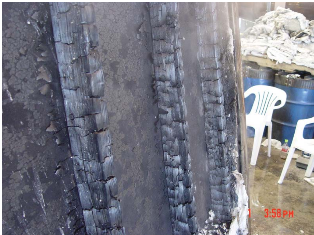
Photograph 10: Closer view of studs post-test
