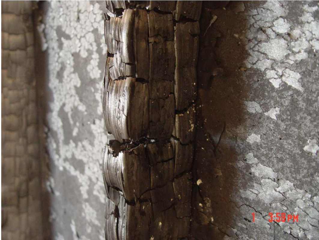
Photograph 11: Close-up of stud post-test
