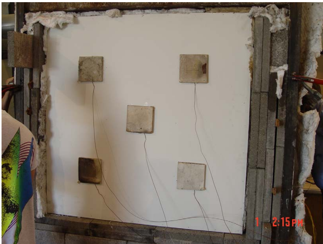
Photograph 2: Sample unexposed face pre-test, showing thermocouples
