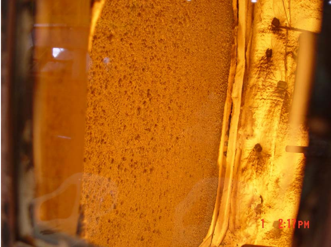
Photograph 3: Sample exposed face beginning to intumesce
