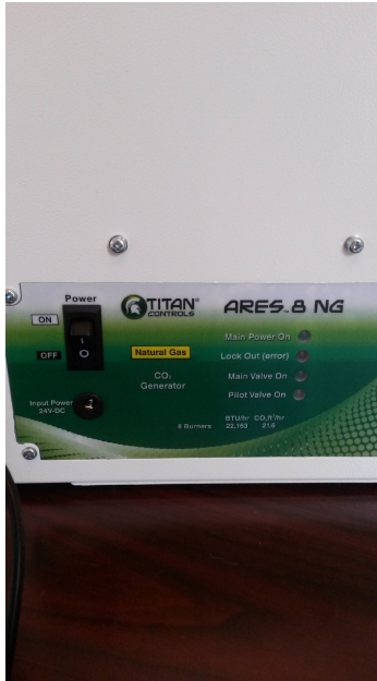
Photo Detail 5 – Unit control panel – front of unit
