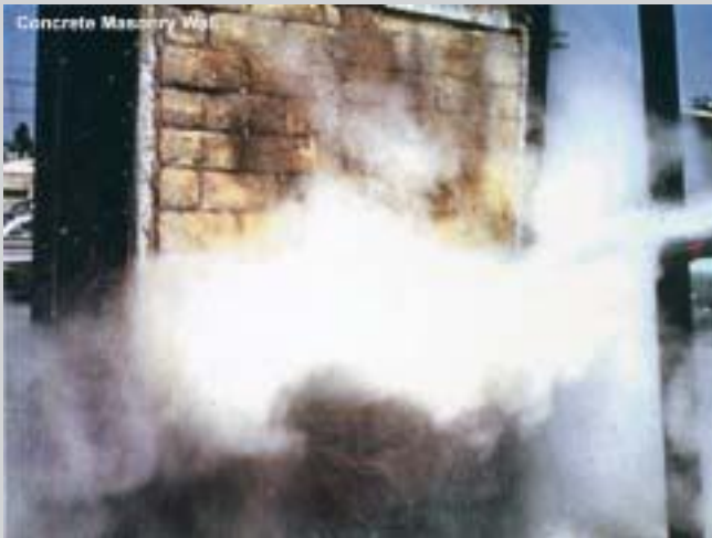
Figure 3. By virtue of duplicate test specimen provisions in ASTM E119 - these are both 2-hour rated walls.
