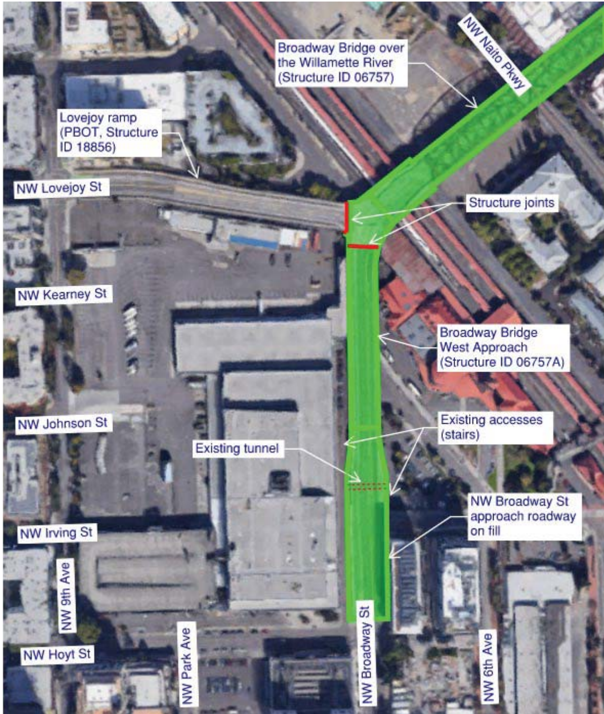
Figure showing areas of concern related to Multnomah County Broadway Bridge (green highlighting), existing Bridge Approach Easement not shown.
