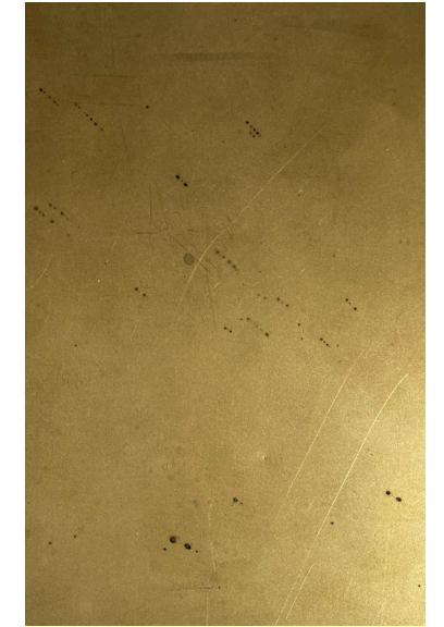
Copper with Bead Blasted Finish Custom Vertical Fins (East / West Levels 2-5)
