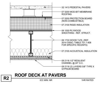
There is no test of this exact assembly, but based on our professional analysis of the a base assembly, plus modifiers as discussed below, the assembly exceeds the STC 50 and IIC 50 minimums.
